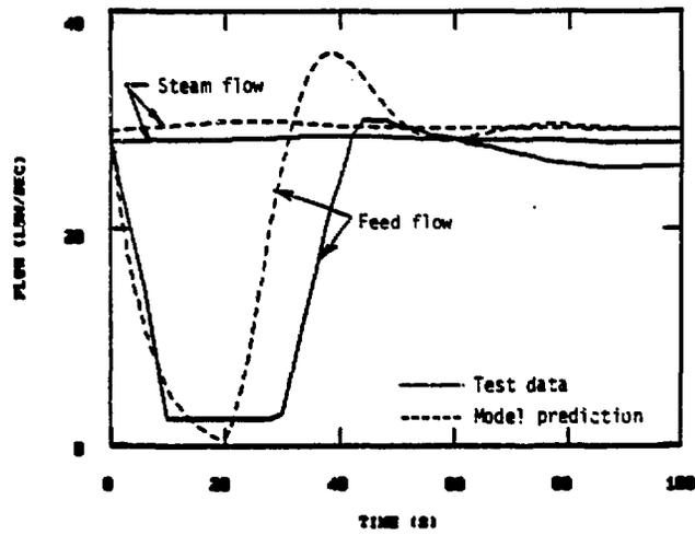
Figure 3. Steam generator level setpoint decrease, 50% power
