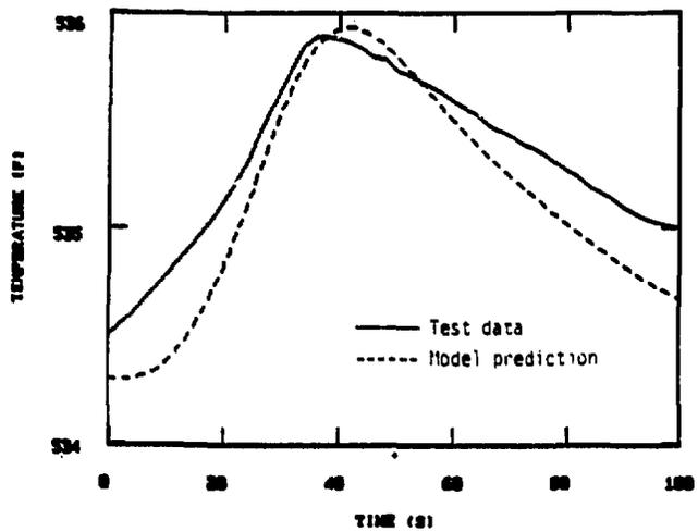
Figure 4. Steam generator level setpoint decrease, 50% power
