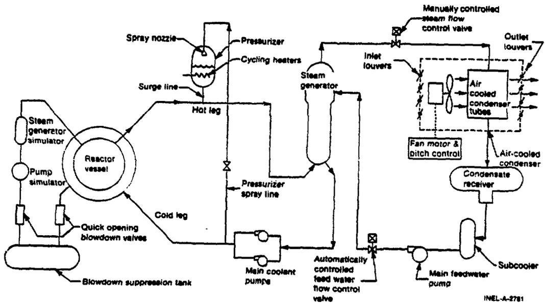
Figure 1. LOFT reactor plant schematic diagram
