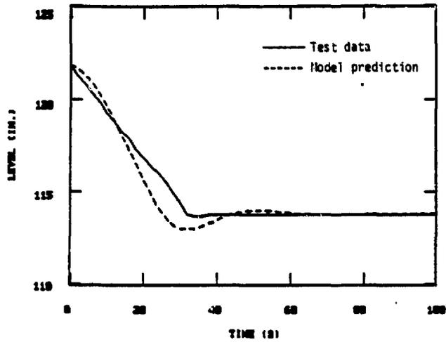
Figure 2. Steam generator level setpoint decrease, 50% power
