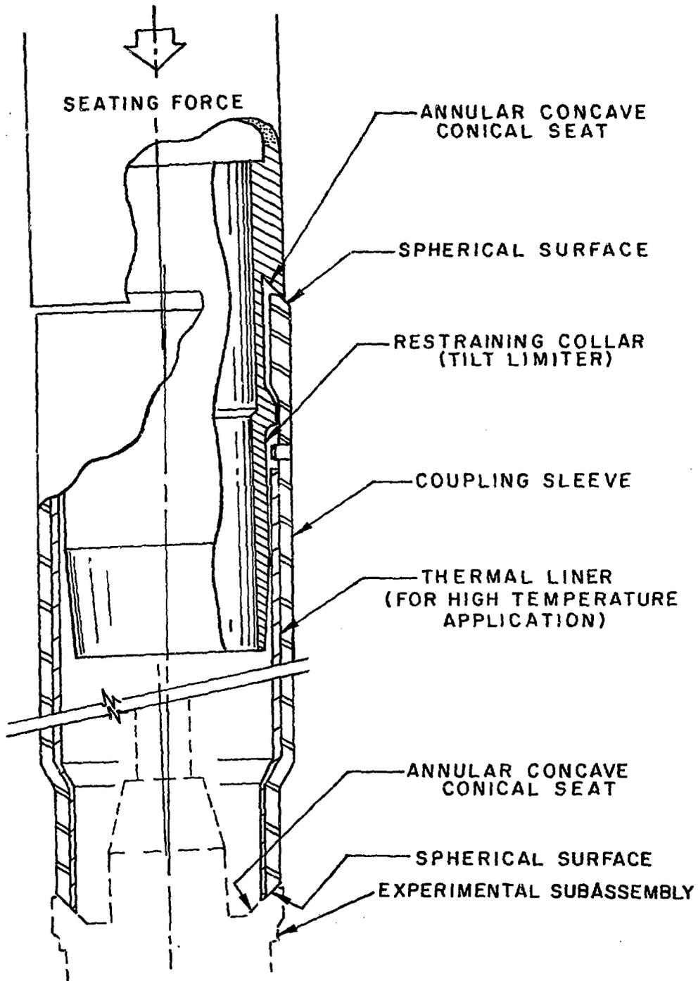
FIG. 2 SEALING COUPLING
