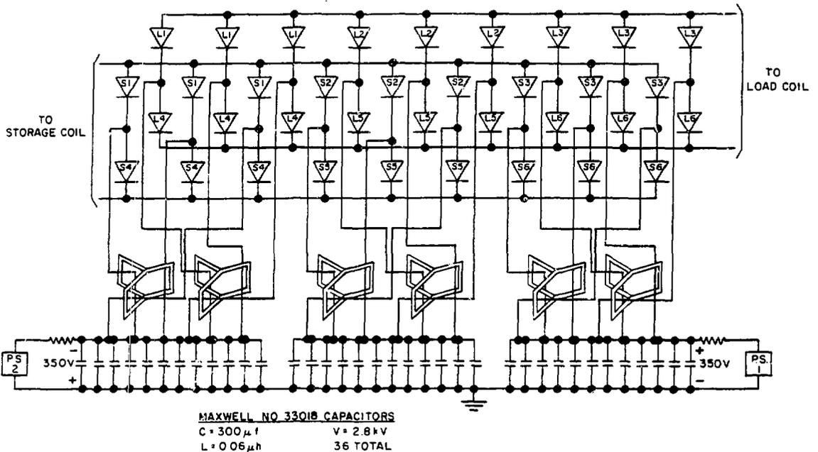
Fig. 3. Circuit diagram for a 5 kA ICB with thyristor current equalizing
