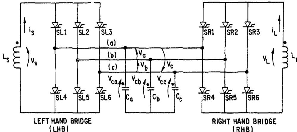
Fig. 1. Circuit Diagram for the 3-Capacitor Model IC Bridge.
