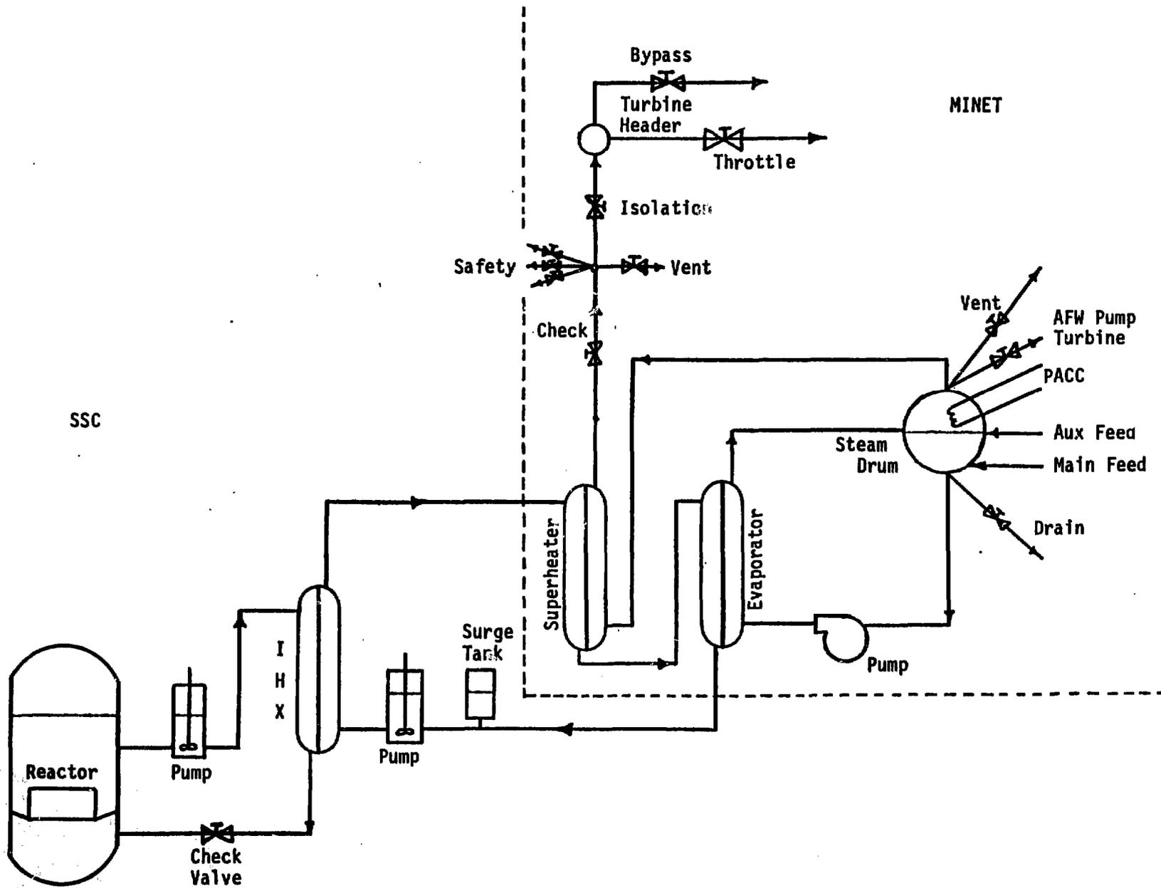
Figure 1. Clinch River Breeder Reactor Plant (CRBRP) Representation Using SSC/MINET
