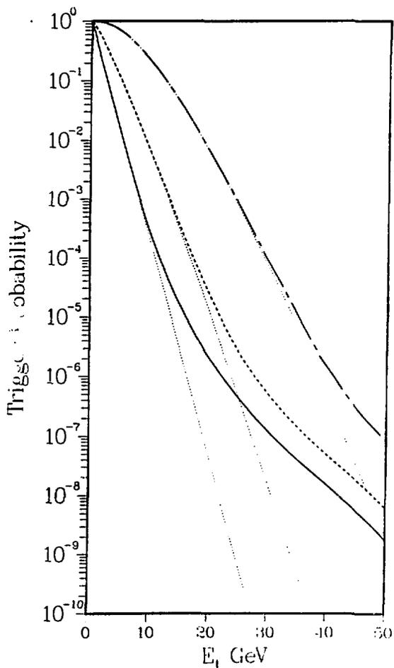
Figure 2. Trigger probability per interaction for the cross section  $P_0^0(E) = .84 e^{-.64E}$  for  $E < 10$  GeV and  $P_0^0(E) = 1.8 \times 10^4 \cdot E^{-8}$  for  $E > 10$  GeV. Solid line is the integral production cross section, dashed line for  $n = 1$  and dashed-dotted line for  $n = 5$ . The dotted lines are the curves from Figure 1 for the pure exponential distribution.
