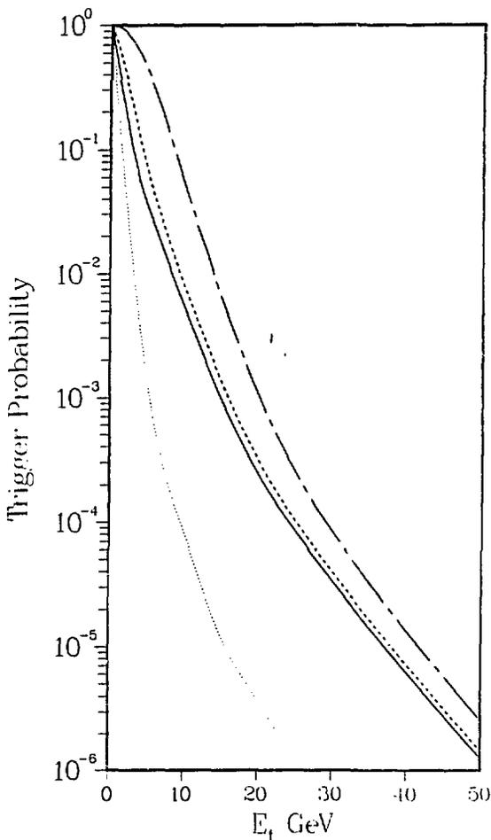
Figure 4. Trigger probabilities per interaction for the reduced solid angle trigger described in the text. The solid line is the integral production cross section used for  $P_0(E)$ ; the dotted line is the random jet probability distribution used for the convolution integrals. The dashed curve is for  $n = 1$  and the dashed-dotted curve for  $n = 5$ .
