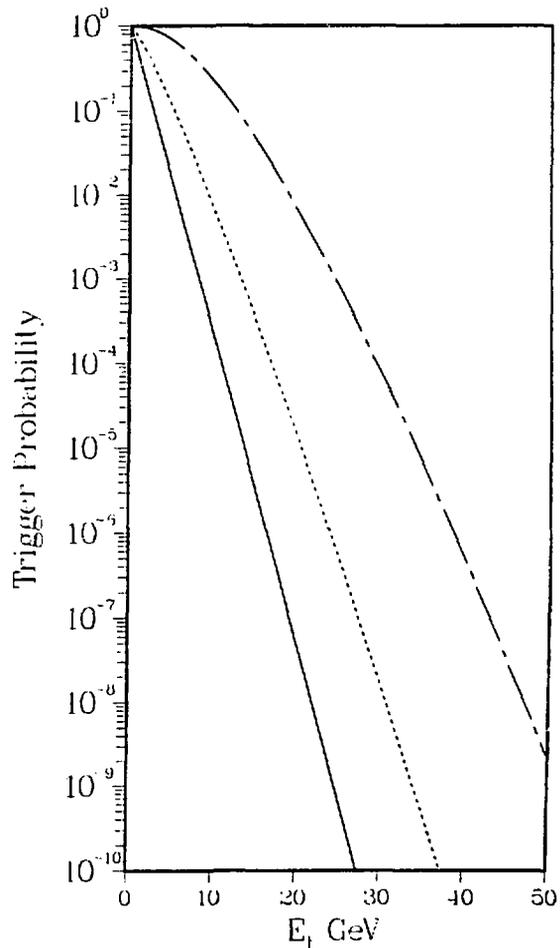
Figure 1. Trigger probability per interaction for the cross section  $P'_0(E) = .84 e^{-.84 E}$ . Solid line is the integral production cross section ( $n = 0$ ). Dashed line is for  $n = 1$  and dashed-dotted line for  $n = 5$ .
