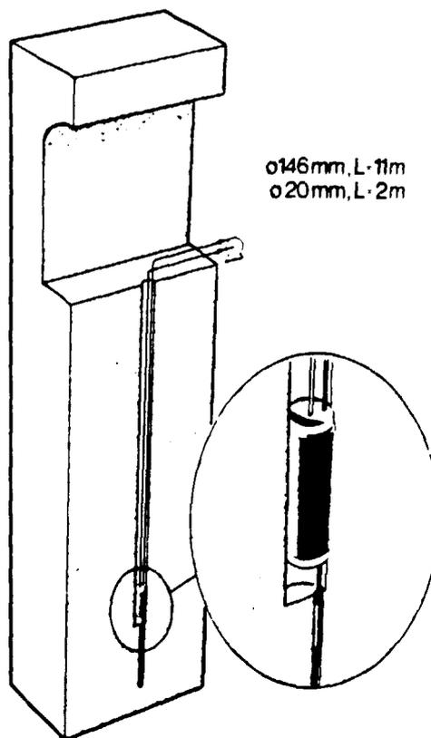
Figure 3. Drilling dimensions and packer positions
