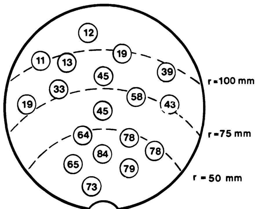
Figure 9. Concentration distribution for Cr-EDTA in the sampling cores from piece No. 10. The numbers represent the relative concentration in per cent.
