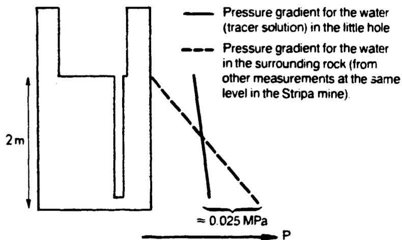
Figure 4. Pressure gradients for injection hole and surrounding rock
