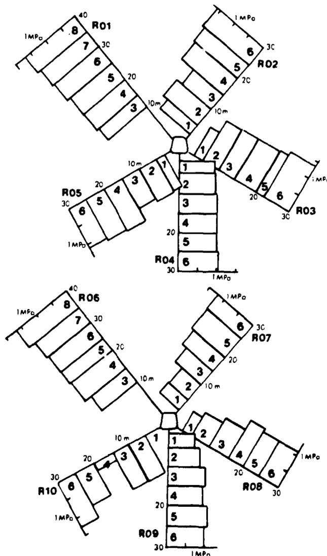
Water pressure in the R-holes in the ventilation drift.
