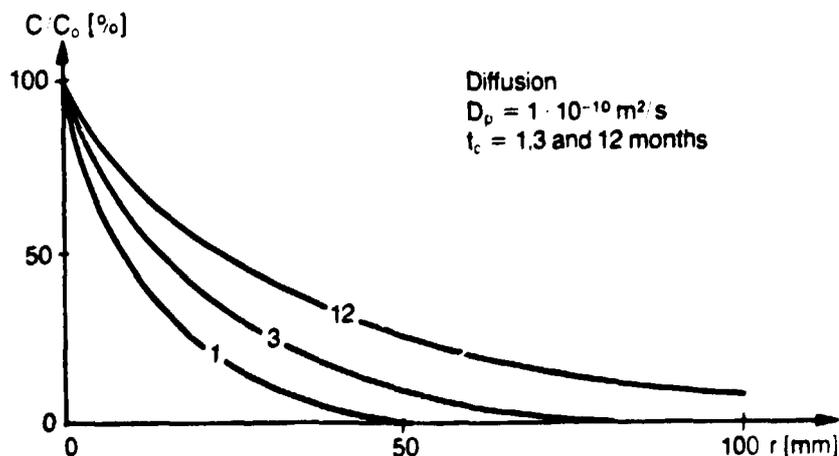
Diagram 2. DIFFUSION.  $c/c_0$  vs  $r$ , for various contact times
