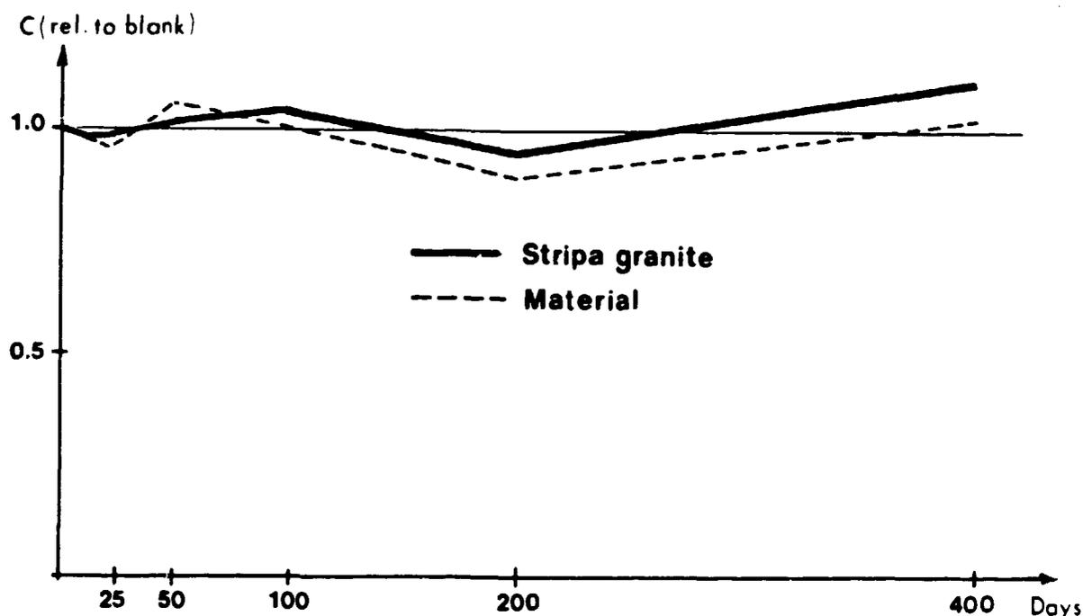
Diagram 7. Sorption test on I<sup>-</sup>. c (relative to blank) vs time.
