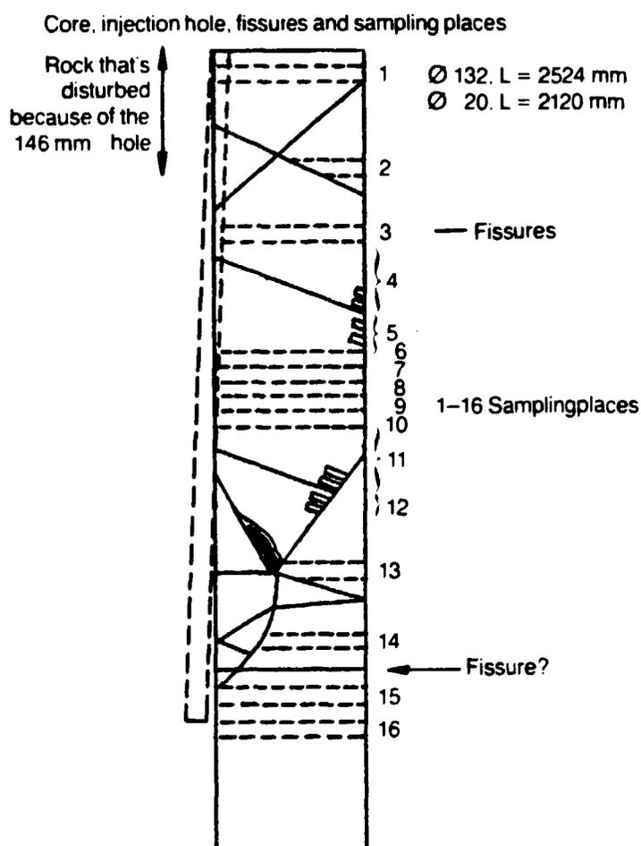
The core from the overcoring of the injection hole was intersected by several fissures. Since there was an inflow of water into the little hole (see chapter 4), at least one of them must have been waterbearing.
