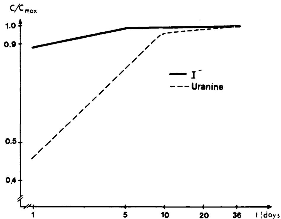
Diagram 6. Leach rate for sampling cores.  $c/c_{\text{maximum}}$  vs time, for  $I^-$  and Uranine.
