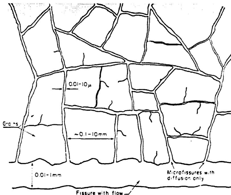
Figure 1. A twodimensional view of the microstructure in granite showing "typical" sizes of grains, microfissures and fissures.
