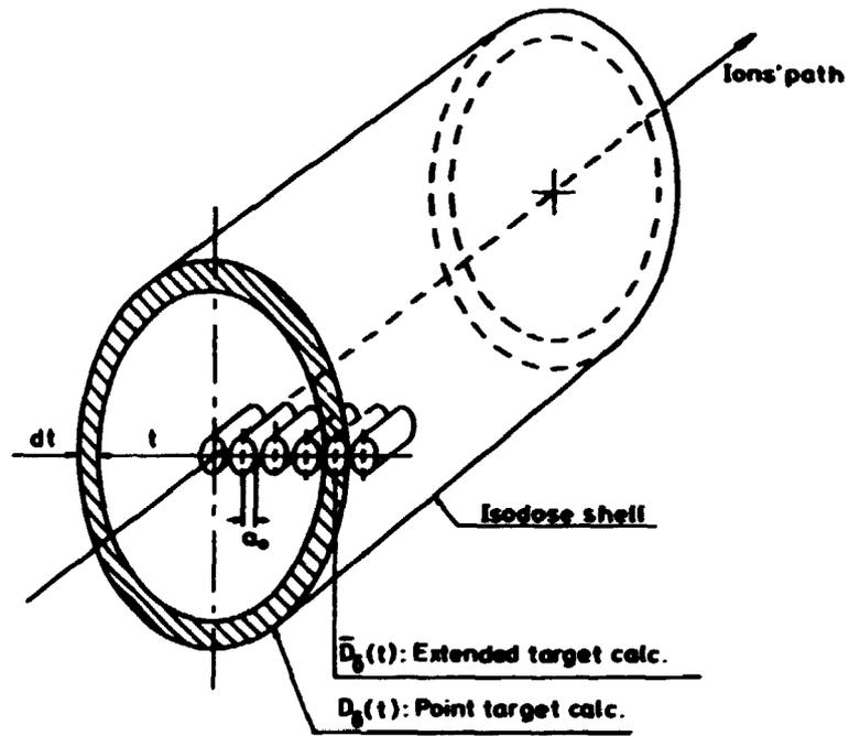
**Fig. 6.** Schematic representation of the radiation sensitive elements around the path of an ion for calculation of the extended target dose.
