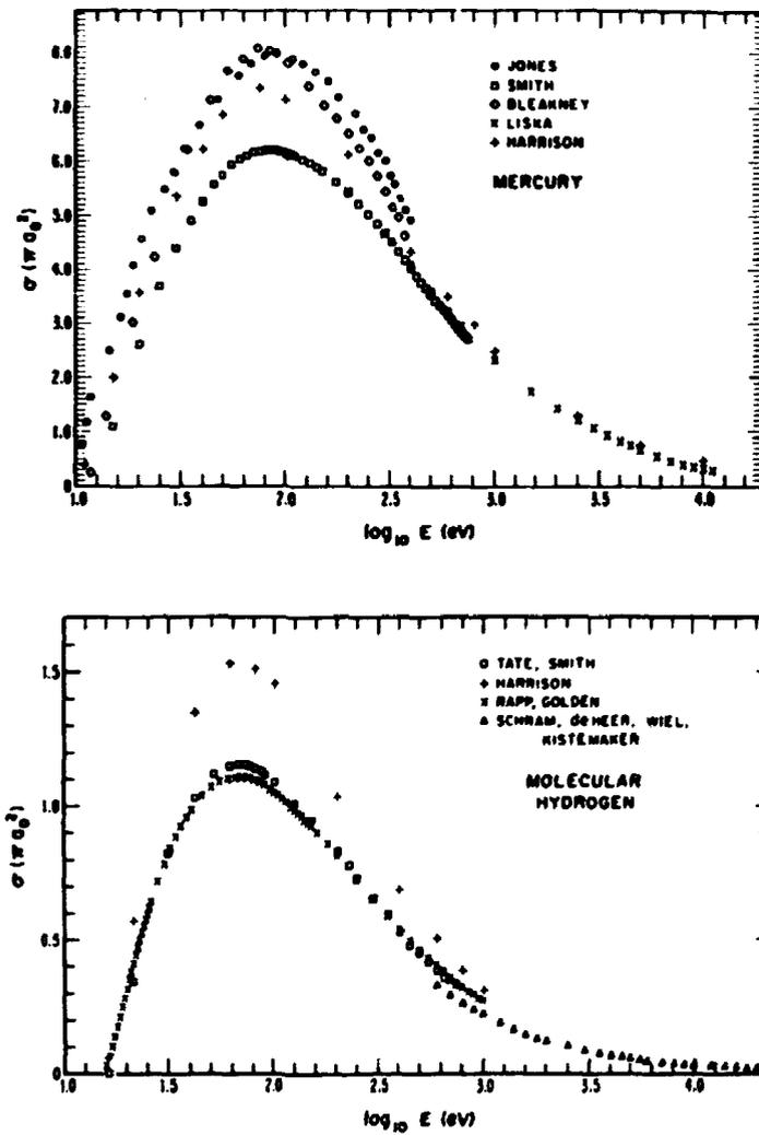
**Fig. 4.** Electron ionization cross-sections of mercury and molecular hydrogen.
