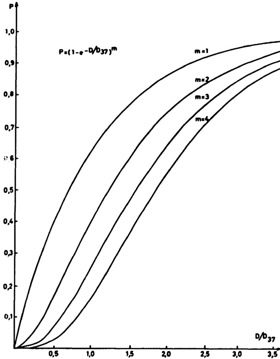
**Fig. 9.** Inactivation probability  $P$  as a function of normalized dose  $D/D_{37}$  with the extrapolation number  $m$  as a parameter.
