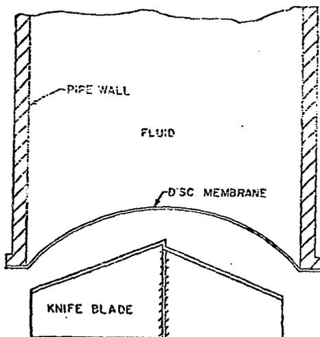
Fig. 1 Reverse Buckling Rupture Disc Design
