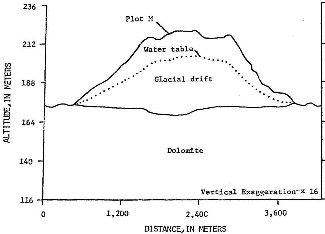
Figure 3. Geologic Cross Section of the Plot M Study Area.
