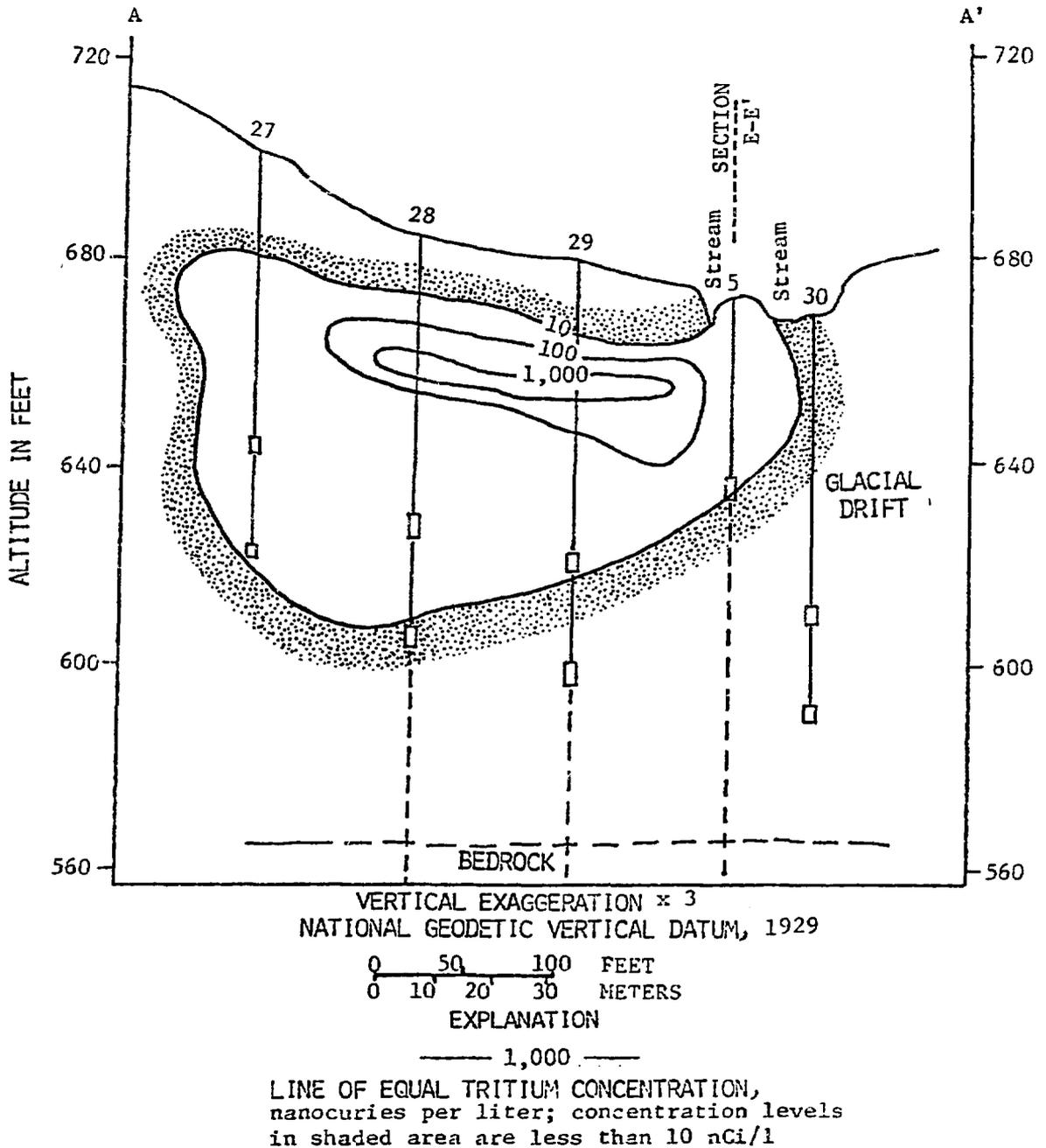
Figure 6. Cross Section A-A'; Leading, Northern Edge of Tritium Plume.
