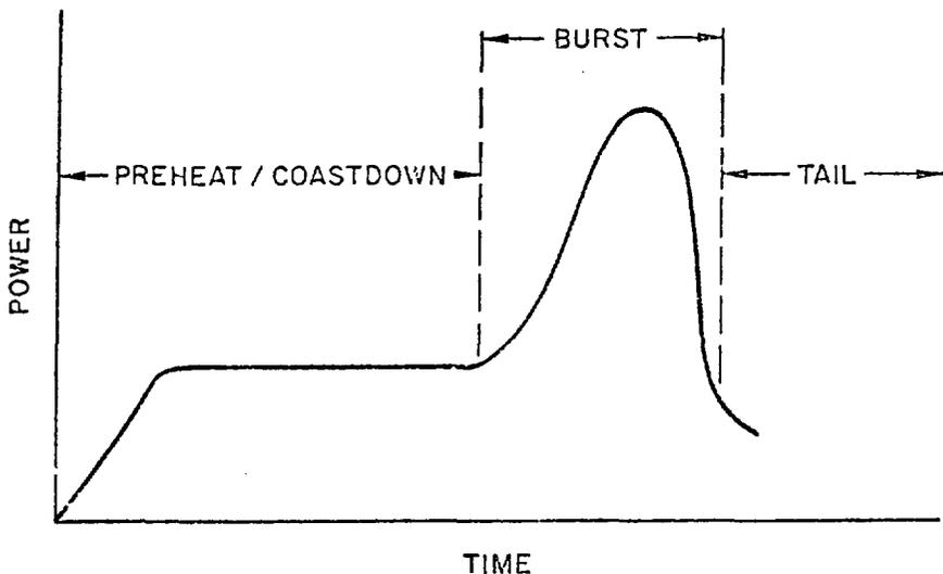
Fig. 1. Transient Shape Definition
