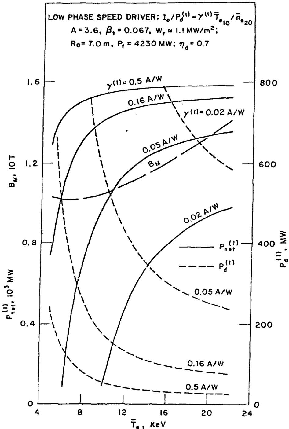
Fig. 8. Driver power and reactor net power for low speed driver ( $v_1 < v_e$ ) and various efficiency coefficients.
