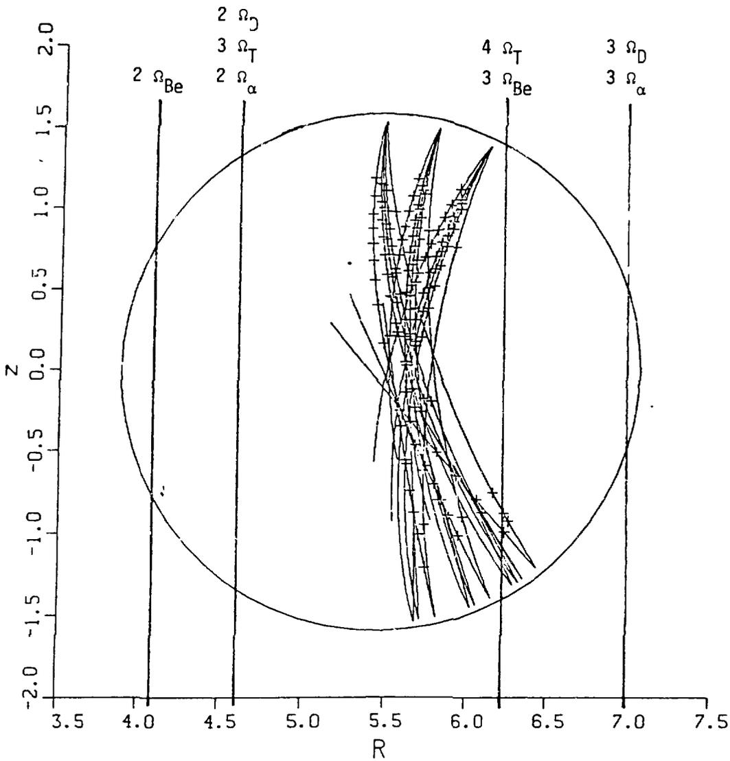
Fig. 4. Typical HSMS ray trajectories;  $\bar{T}_e = 12$  keV.
