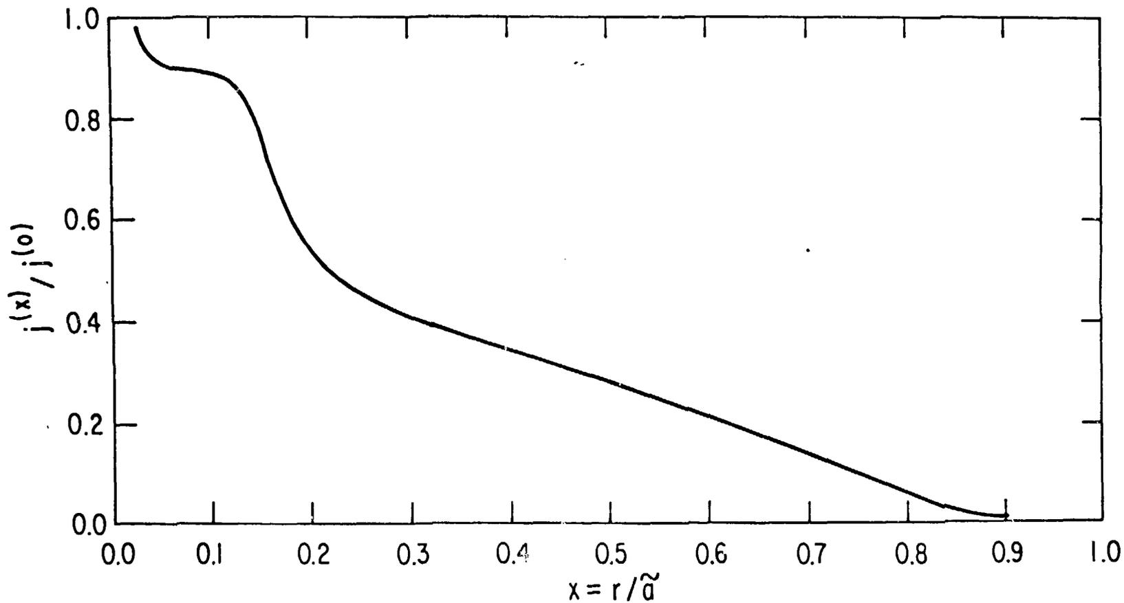
Fig. 5. Current density profile for HSMS at 82 MHz and  $\lambda_{\perp} \approx 0.8$  m;  $\bar{T}_e = 16$  keV.
