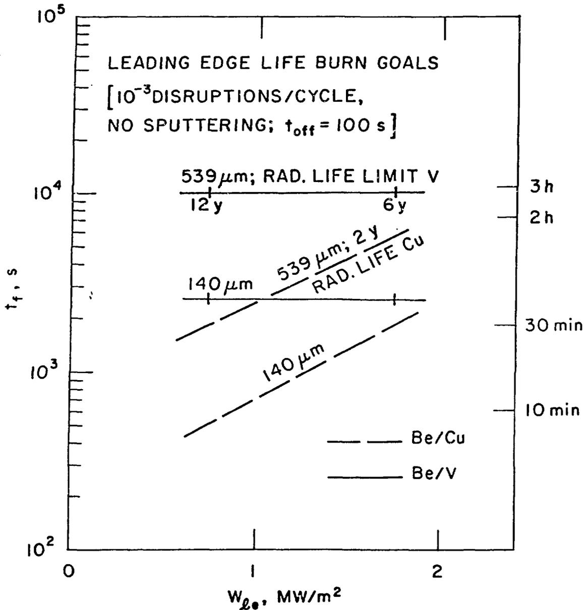
Fig. 10. Minimum burn periods required such that cyclic effects (from thermal fatigue and disruption damage) are less life limiting than radiation damage. Disruption damage is parameterized by moderate (140  $\mu\text{m}$ ) and severe (539  $\mu\text{m}$ ) beryllium losses per disruption.
