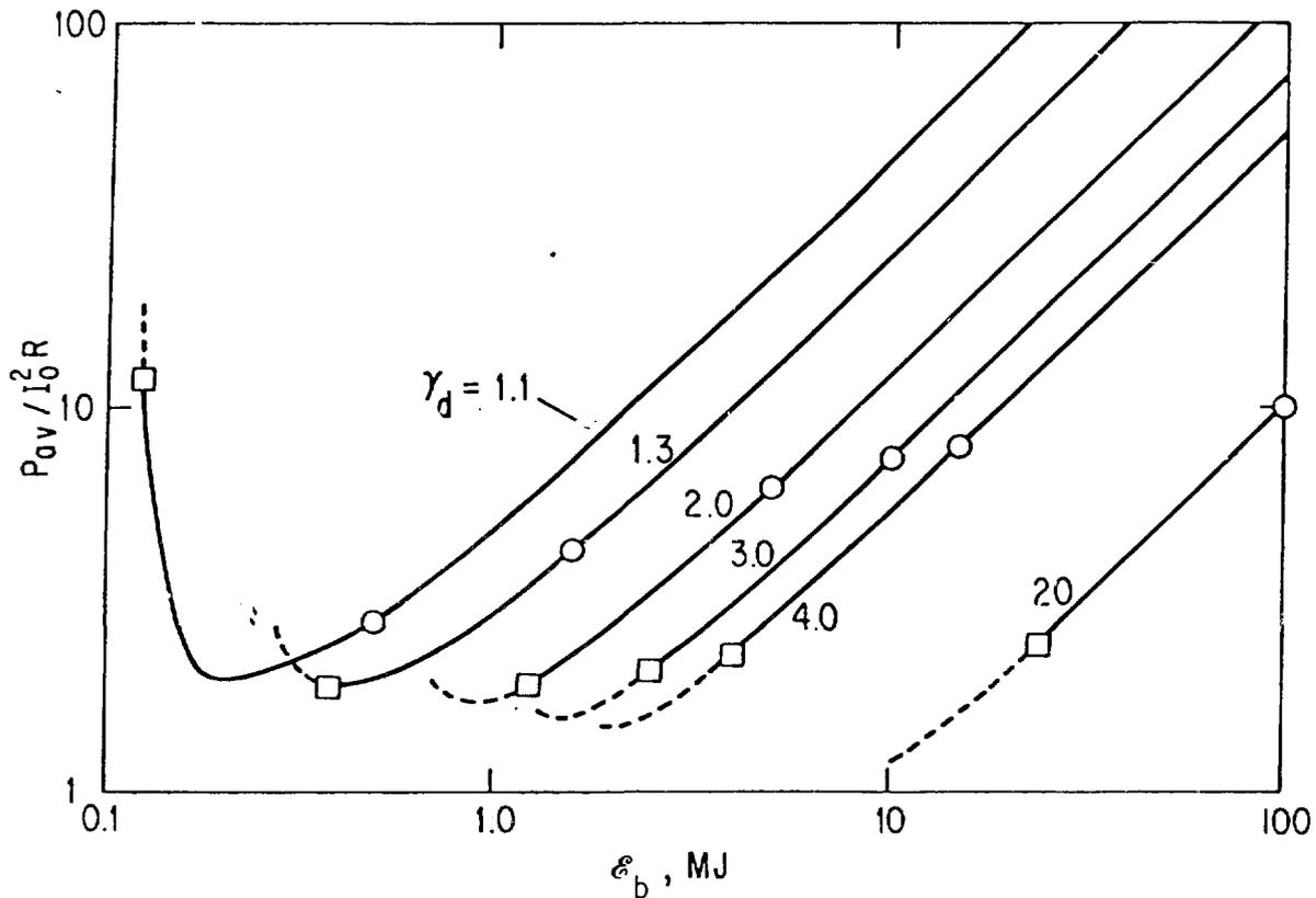
Fig. 6. DEMO with  $R_0 = 5.2$  m,  $I_0 = 9.01$  MA; analytic theory is valid between boxes and circles. Time average REB power is given in terms of relativistic  $\gamma_d$  at the diode and total beam kinetic energy,  $\mathcal{E}_b$ , in the pulse.
