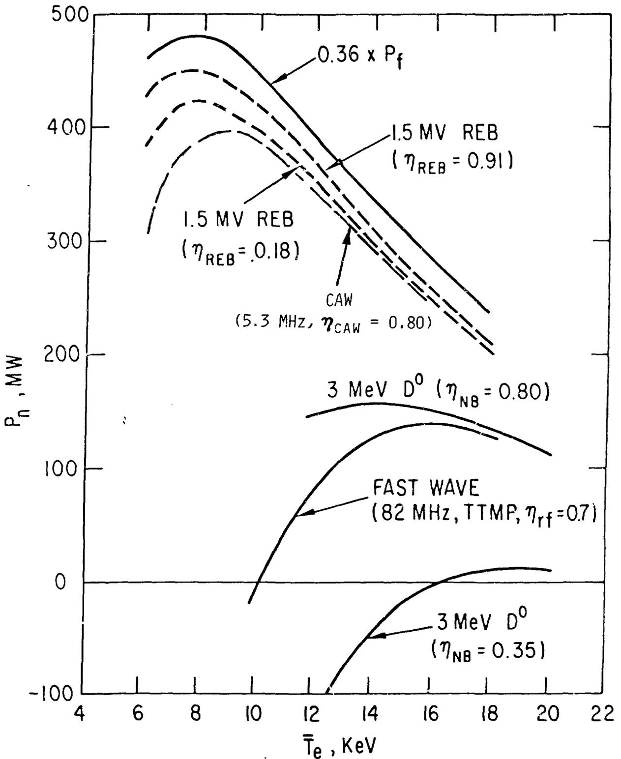
Fig. 3. Net electric power for DEMO with different current drivers.
