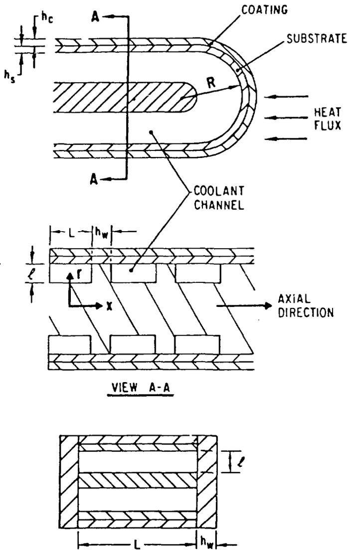
Fig. 9. Leading edge geometry used for stress calculations in limiter; INTOR model.
