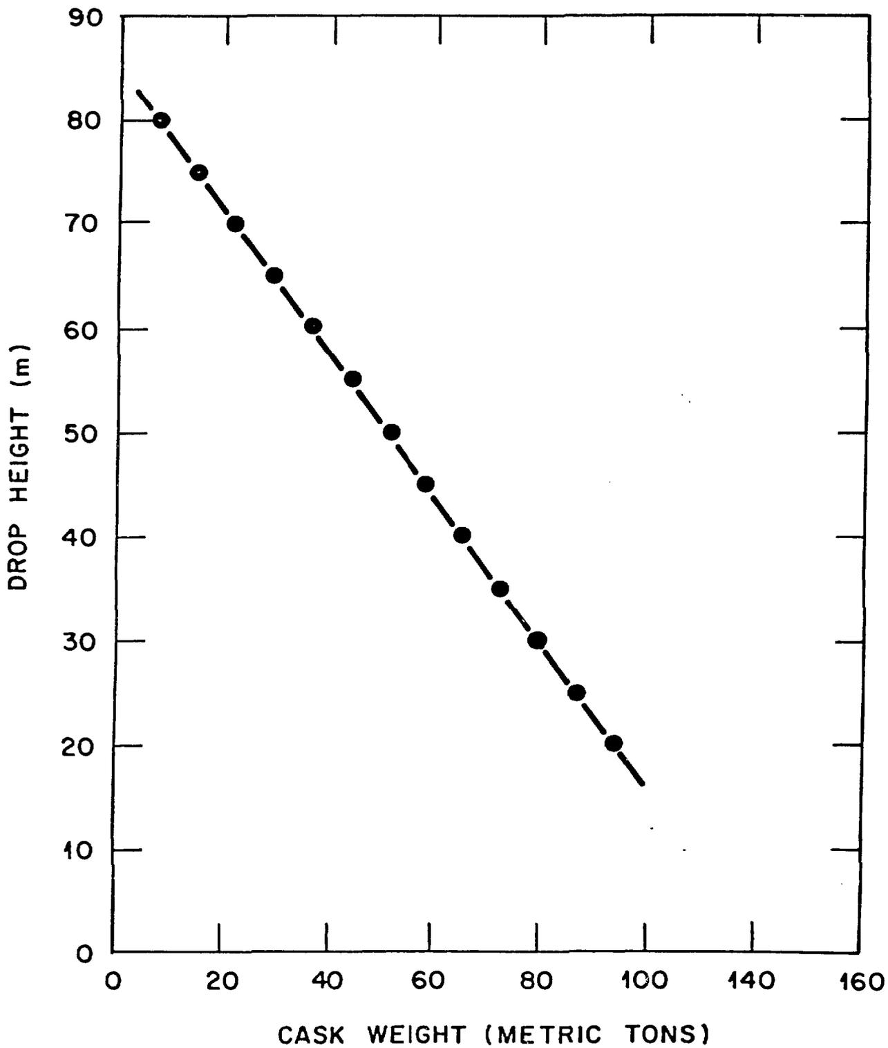
Fig. 2. Tower Lifting Capacity vs Drop Height.
