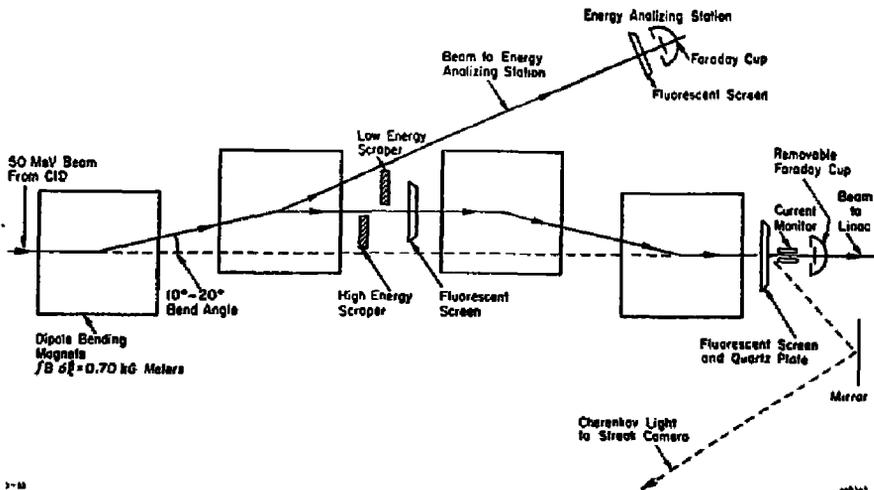
Fig. 5. Bunch Compressor.
