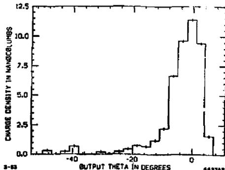
Fig. 4. Calculated Charge Distribution with  $7.5 \times 10^{10} e^-$ /bunch  $\sigma_s = T^0 = 7$  psec.
