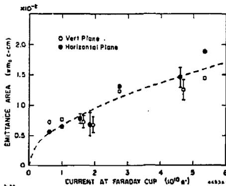
Fig. 6. Emittance versus Current. Error bars at  $\pm \sigma$ . Where no error bars are shown there is insufficient data to determine  $\sigma$ .
