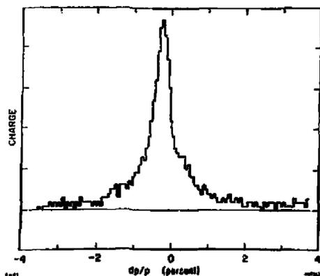
Fig. 2. Injector Momentum Spectrum.
