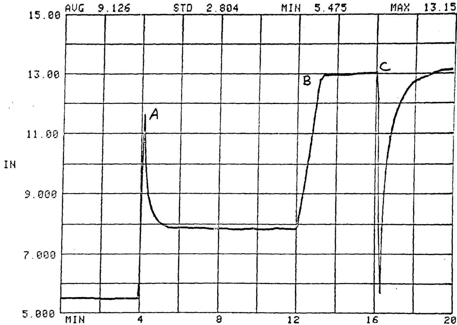
FIG. 3 ROD POSITION FOR ACADS TRANSIENT.
