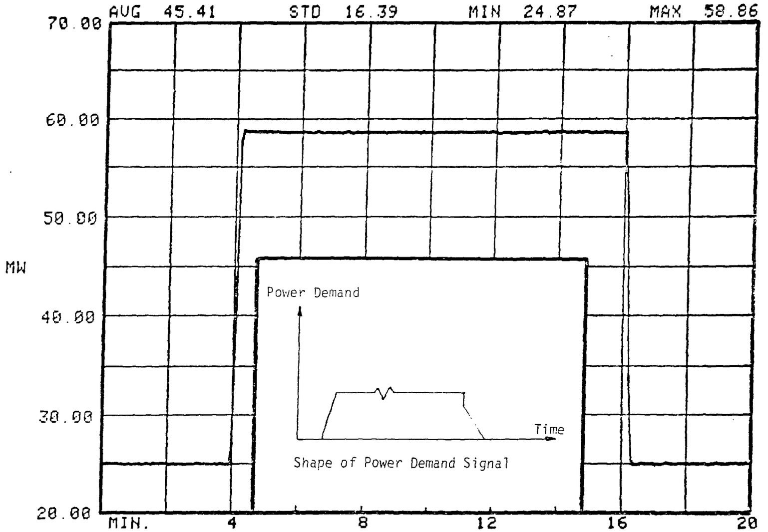
FIG. 2 POWER RESPONSE AND DEMAND SIGNAL SHAPE FOR AC RDS TRANSIENT.
