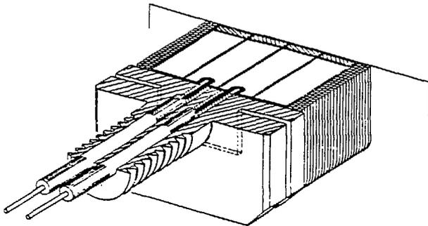
As shown, one of the stud heads is bonded to the SiGe thermopile, while the other bears against the aluminum housing wall. The intervening stress-relief slots (from all four edges) effectively serve to isolate the thermopile from the effects of the aluminum wall expansion.
