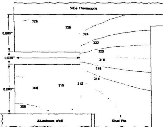
As can be seen, the temperature drops for the dimensions shown in Figure 11 are considerable but not prohibitive. Therefore, these dimensions were tentatively selected for the stress analysis required to evaluate the merit of the concept.
