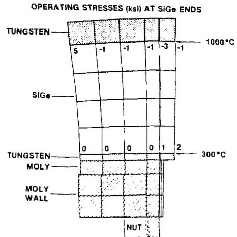
As can be seen, the high operating stresses near the center of the cold end virtually vanish when the expansion coefficient of the wall matches that of the cold stud.
