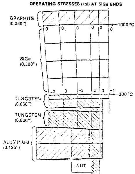
Table 8 compares the cold-end stresses for single-headed and double-headed cold studs. As can be seen, the double-headed stud has slightly higher fabrication stresses, as the result of its greater thickness and stiffness. But its peak operating stress is only one fifth that of the single-headed stud.
