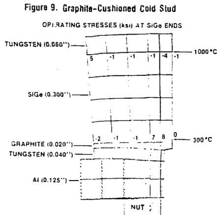
As can be seen, the graphite layer is quite compliant. As shown in Table 6, its use completely eliminates the cold-end fabrication stresses, and cuts the cold-end peak operating stress in half. While this was not considered good enough to ensure survival by itself, it was a big step forward and its use is beneficial in conjunction with other design improvements, as shown in Sections 6.2 and Reference [4].
