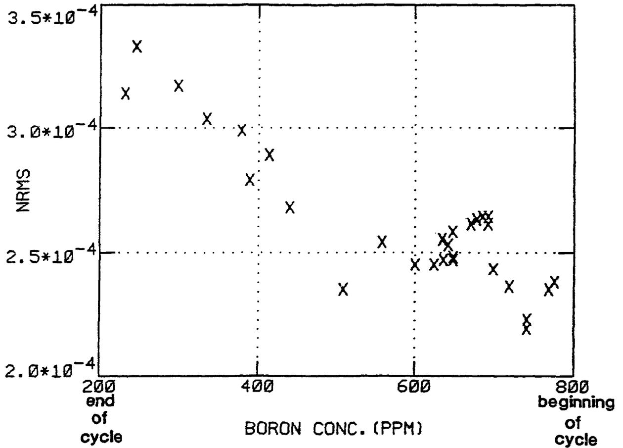
Fig. 1. Measured normalized root mean square (NRMS) of ex-core neutron detector noise over 2.0 to 4.0 Hz at Sequoyah-1 vs soluble boron concentration for the first fuel cycle.
