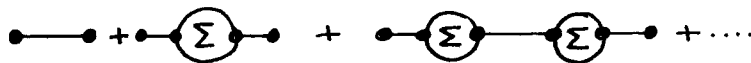
Figure 31 : The dressed electron propagator, where \Sigma is the sum of all one-particle-irreducible self-energy insertions.
