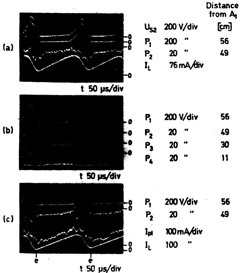
Fig.2. (a) Periodic current disruptions (lowest trace) showing the potential variations of  $S_2$  and of two emitting probes  $P_1$  ( $z = 56$  cm) and  $P_2$  ( $z = 49$  cm), separated by 7 cm ( $z$  is the coordinate measured from  $A_1$ ). The inductive voltage (350 V) appears as a potential drop across a double layer in the plasma between  $P_1$  and  $P_2$ . The zero levels are marked in the same order as the traces.  $U_0 = 100$  V,  $I_{pl} = 105$  mA.
