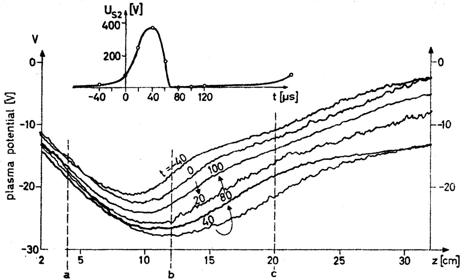
Fig.3. Potential profiles along the axis in the left part of the experimental chamber at times before, during and after a disruption. The times are indicated by open circles in the inserted oscillogram of a disruption voltage pulse. The curves were obtained by sampled measurements of the floating potential of an emitting probe. Sampled Langmuir probe measurements were made at the points, a, b, c.
