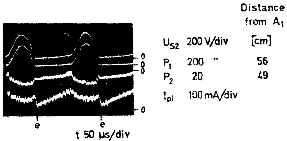
Fig. 6. Oscillograms from an experiment with increased L and C. L = 1.0 H, C = 70 nF. The double layer is maintained during the whole voltage pulse, which has a duration 1.25 times the half period of the undamped LC circuit. U<sub>0</sub> = 100 V.
