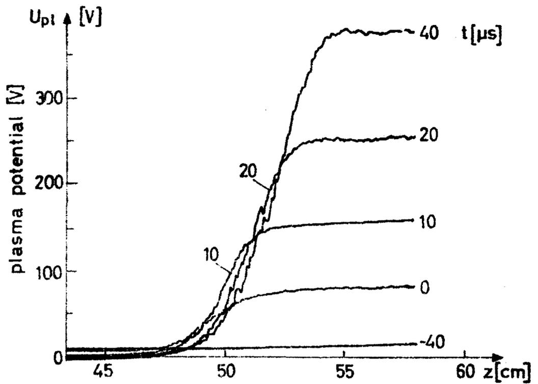
Fig.4. Potential profiles showing the double layer in the right part of the experimental chamber at times before and during the build-up of a disruption (cf. Fig.3). The transition from low to high potential is seen to take place within 5 cm or less.
