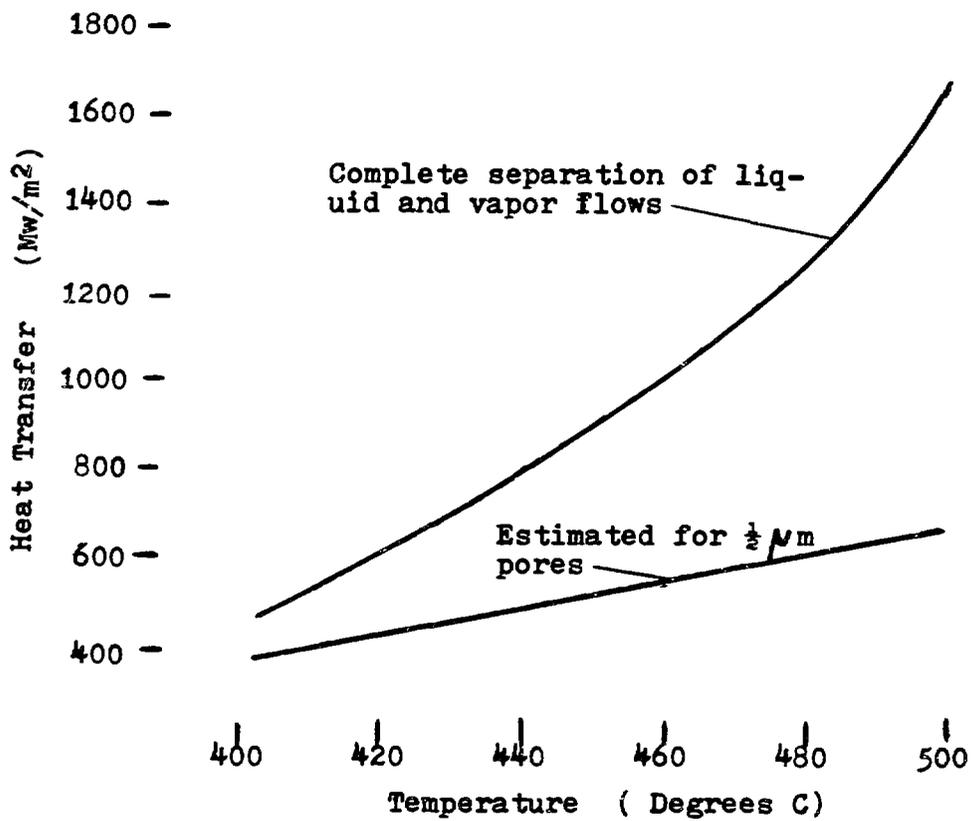
Fig. 3 Heat Transfer Capabilities of Mercury Reflux Capsules
