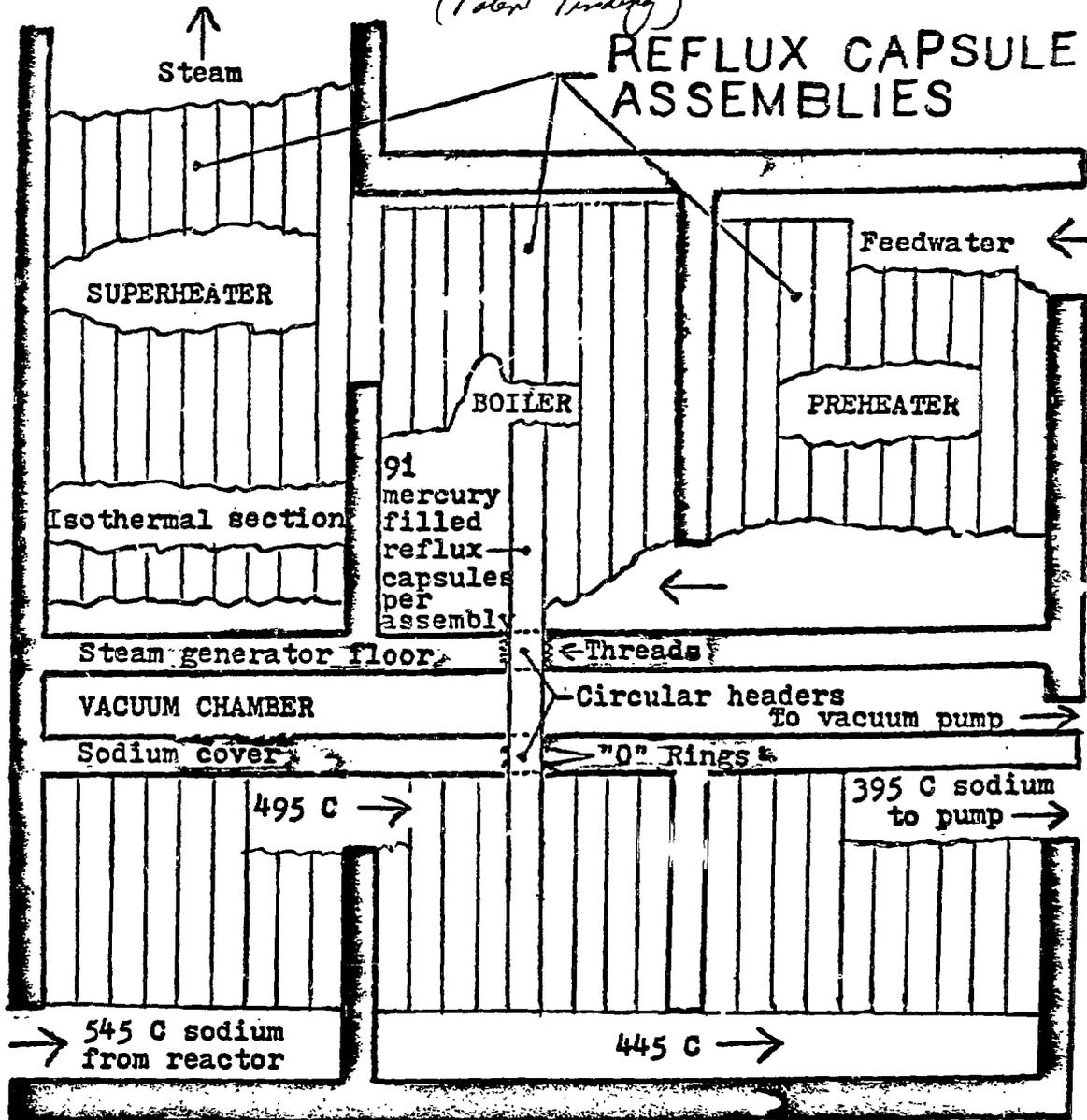
Fig. 8 Flow Schematic for Maximum Steam Temperature
