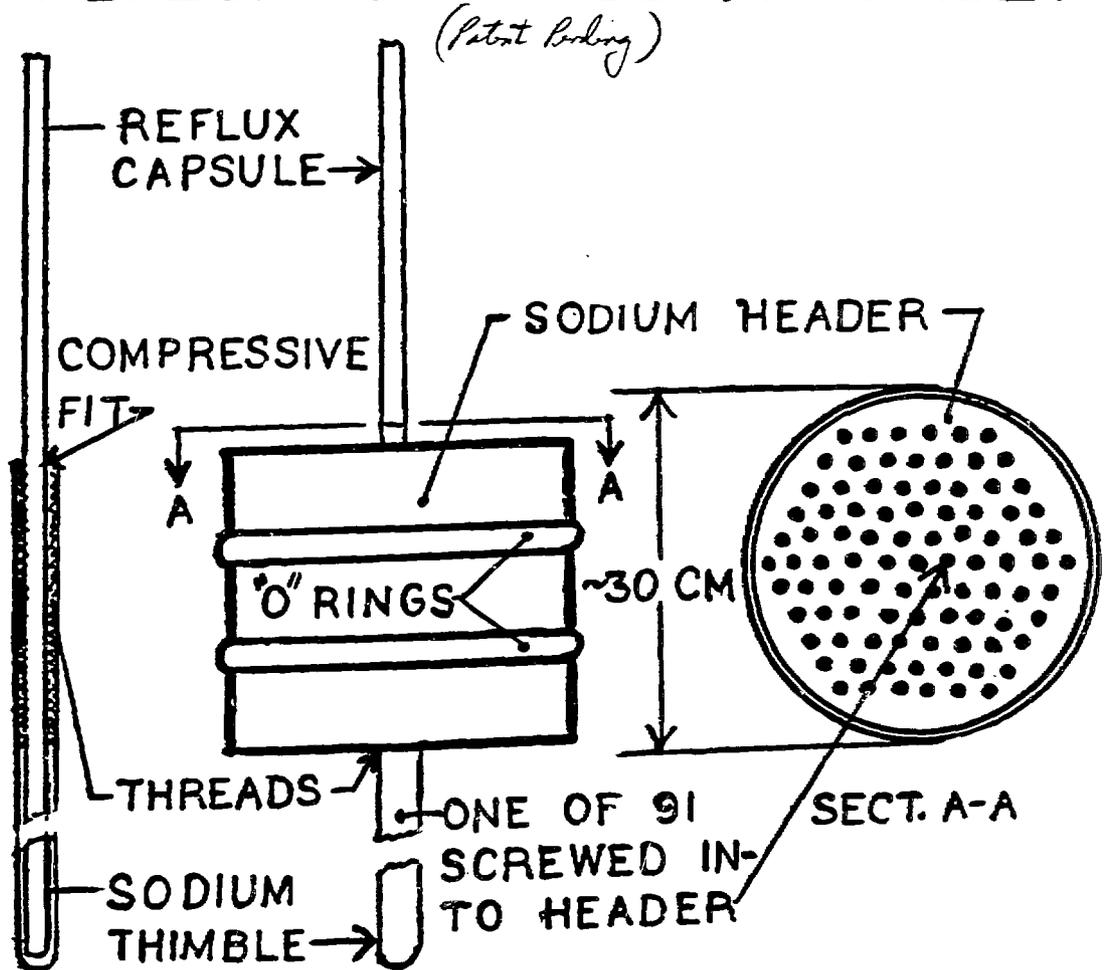
Fig. 5a Sodium Portion of Reflux Capsule Assembly
