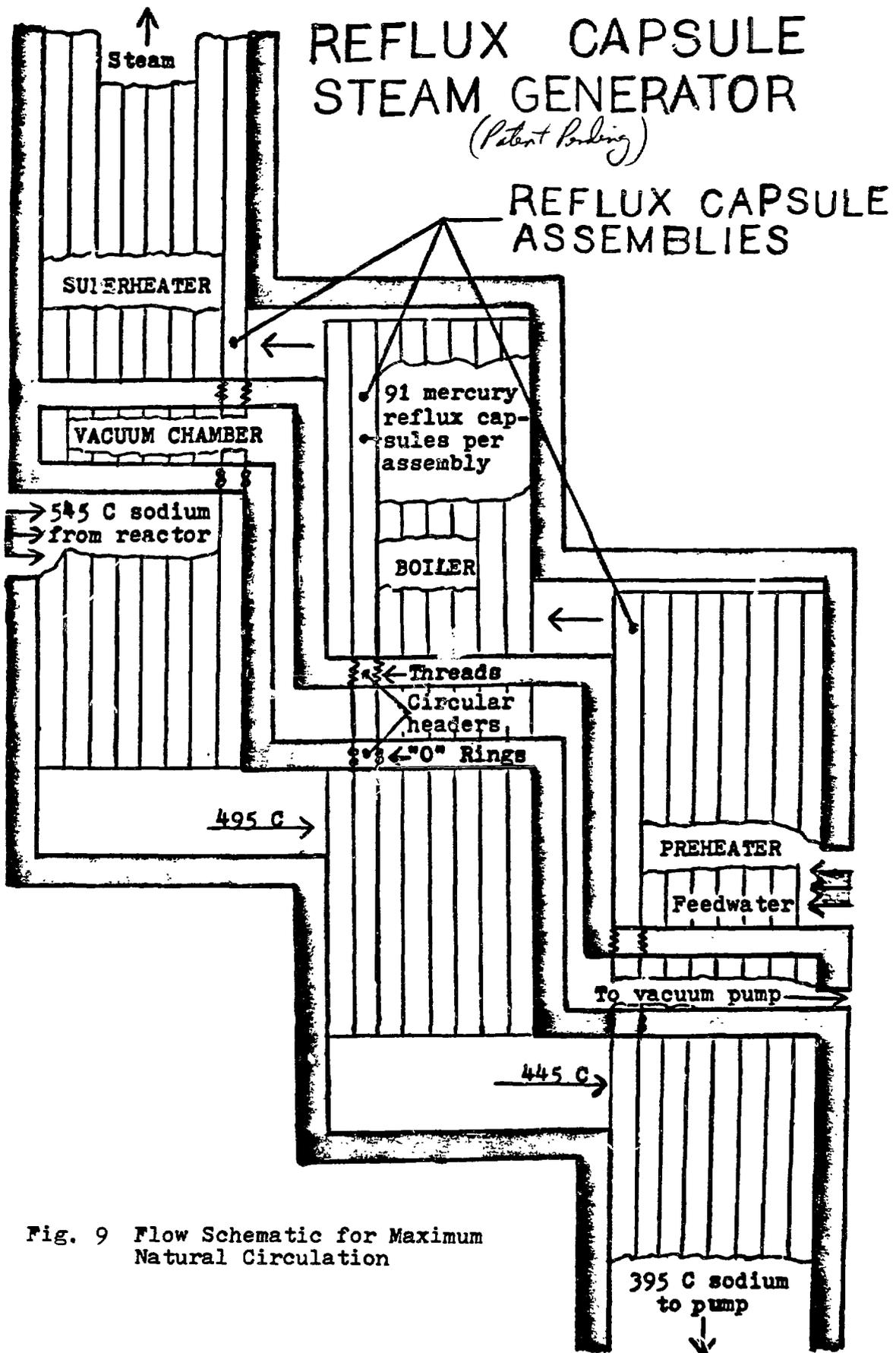
Fig. 9 Flow Schematic for Maximum Natural Circulation
