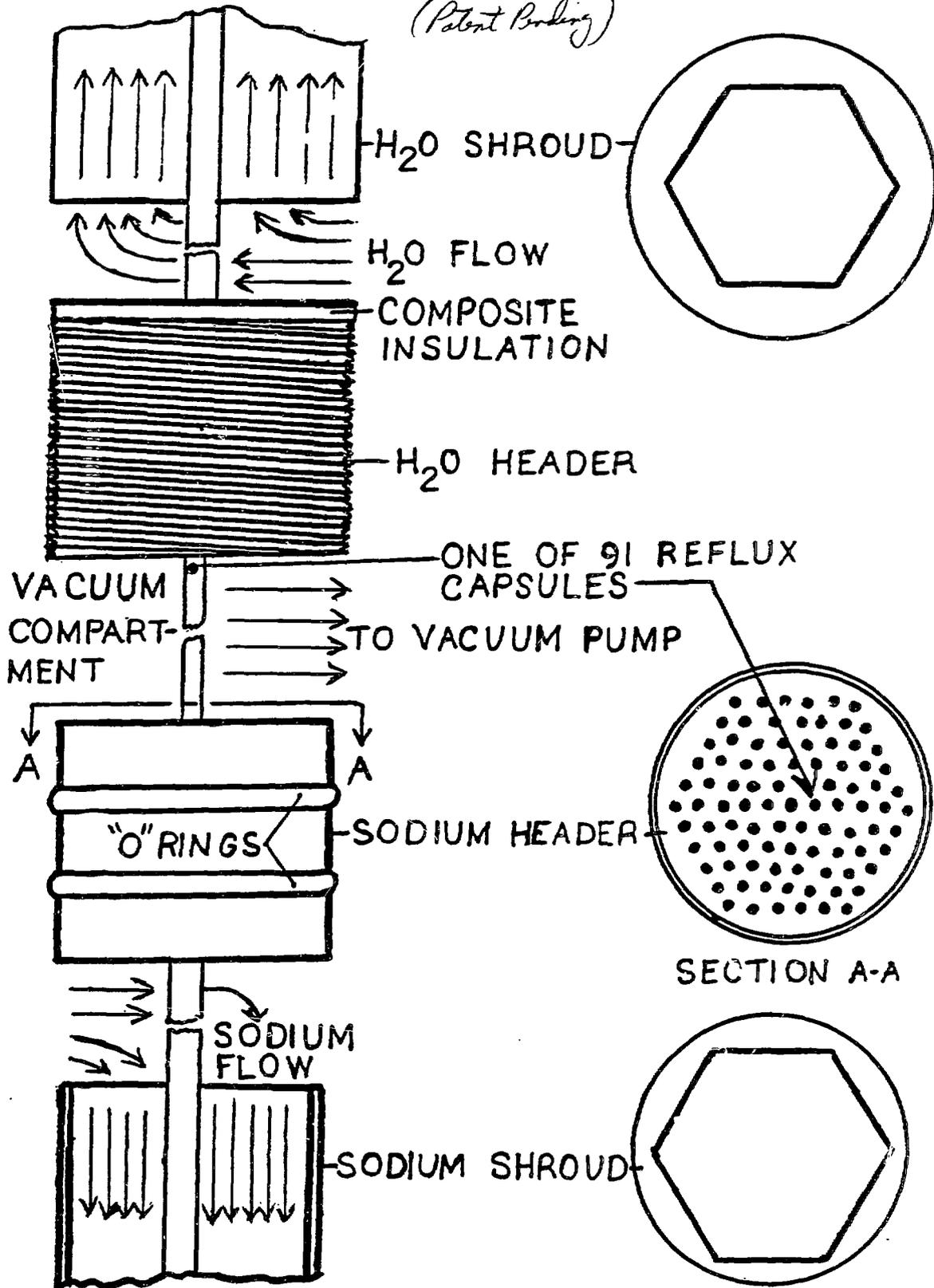
Fig. 6 Composite of Installed Reflux Capsule Assembly
