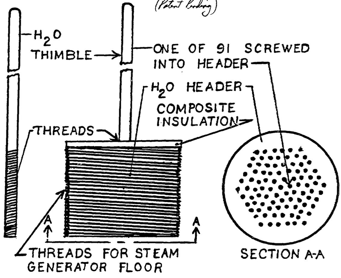
Fig. 5b H<sub>2</sub>O Portion of Reflux Capsule Assembly
