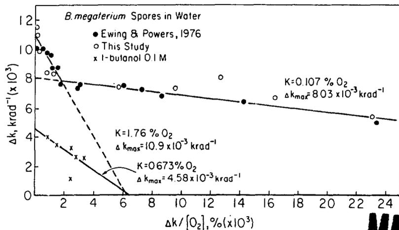
Fig. 1. The dependence of  $\Delta k$  on  $[O_2]$  in bacterial spores presented as the E-H transform.
