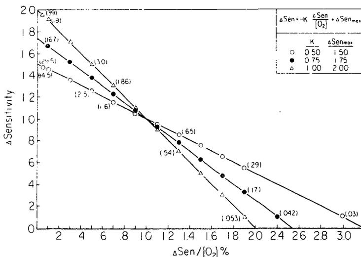
Fig. 8. Hypothetical E-H plots of data with varying K and  $\Delta S_{max}$ . Numbers in ( ) = %O<sub>2</sub>.
