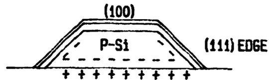
The radiation positive charge created into the sapphire substrate can induce an electron inversion layer in the silicon near the silicon-sapphire interface, connecting source to drain and giving rise to the so called back channel leakage current. [14]
