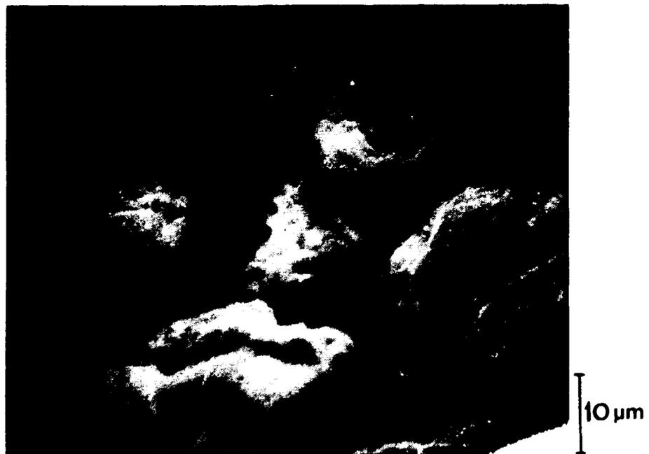
Fig.4. Scanning electron micrograph of dense MX-80 clay "matured" for 1 year. Bulk density  $2.0 \text{ t/m}^3$ .
