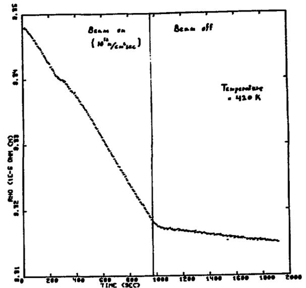
Figure 6. Ordering in  $\text{Cu}_3\text{Au}$  during neutron irradiation (beam on) at 420 K and following cessation of irradiation at 970 sec. Note decay of irradiation-produced vacancy concentration near 1000 sec and evidence for a continuing vacancy diffusion for time  $> 1000$  sec.
