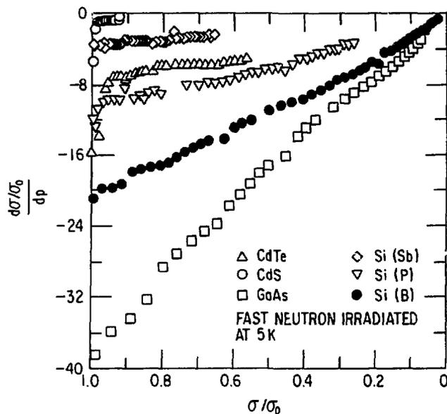
Figure 2. The normalized rate of conductivity change,  $d(\sigma/\sigma_0)/dp$ , vs. fractional normalized conductivity,  $\sigma/\sigma_0$ .
