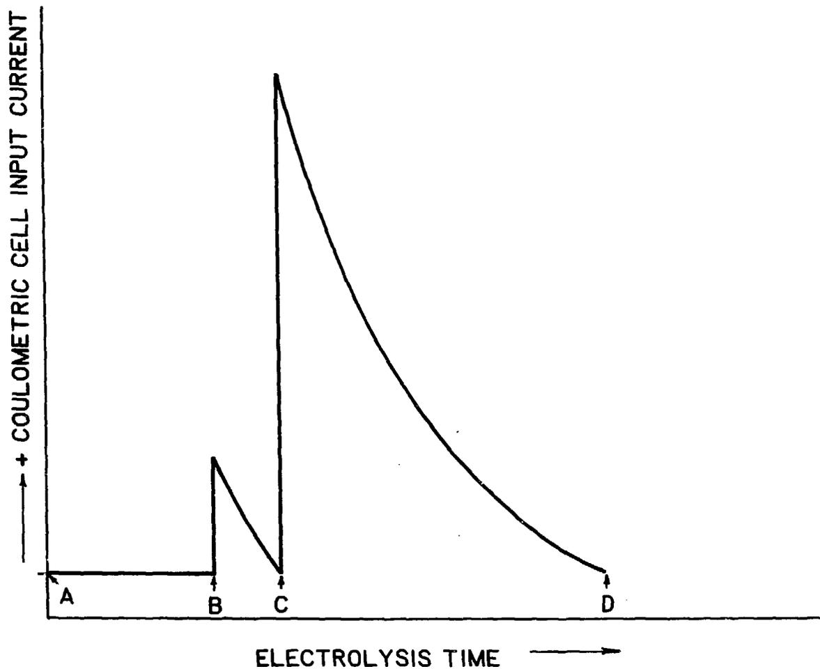
FIGURE 3: SCHEMATIC REPRESENTATION OF COULOMETRIC CELL INPUT CURRENTS DURING DEGASSING (A  $\rightarrow$  B), PRERELUTION (B  $\rightarrow$  C), AND REDUCTION OF A TYPICAL SAMPLE (C  $\rightarrow$  D)
