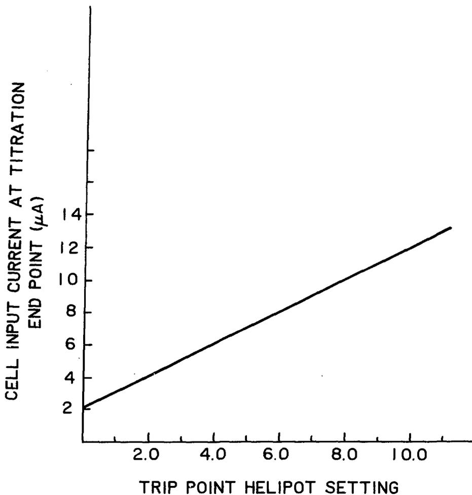
FIGURE 2: TRIP POINT CONTROL HELIPOT SETTING VS. CELL INPUT CURRENT SHUT OFF FOR THE AUTOMATIC MODE OF OPERATION.
