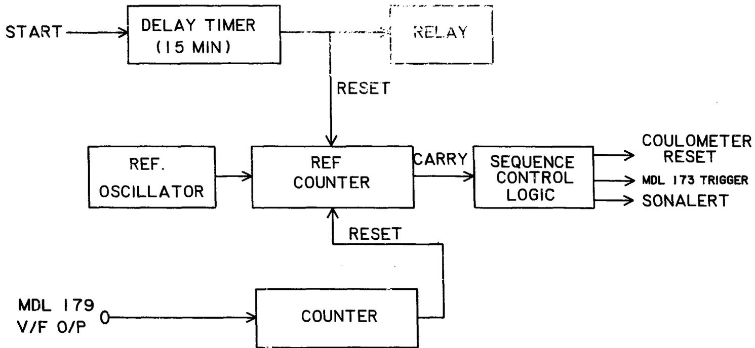
FIGURE 1: SCHEMATIC DIAGRAM OF COULOMETER MODIFICATIONS
