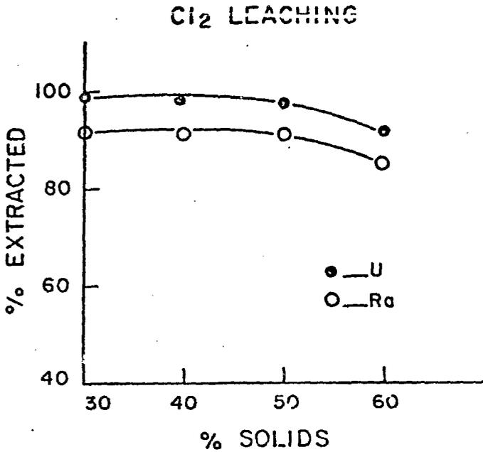
Fig. 4 - U and Ra extraction as a function of pulp density
