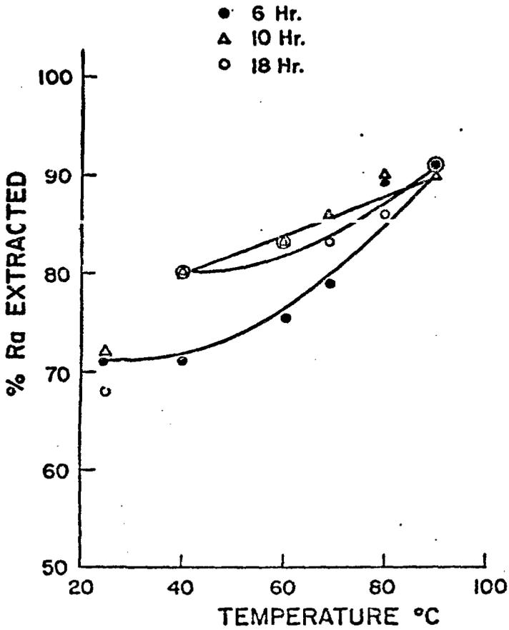
Fig. 2 - Radium extraction as a function of temperature
