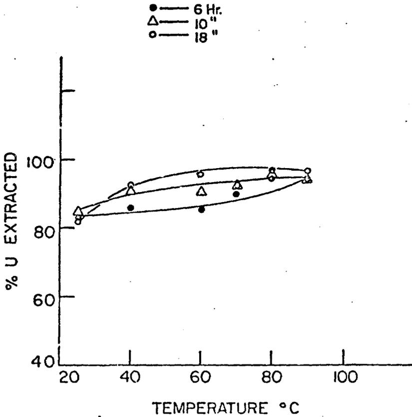
Fig. 1 - Uranium extraction as a function of temperature
