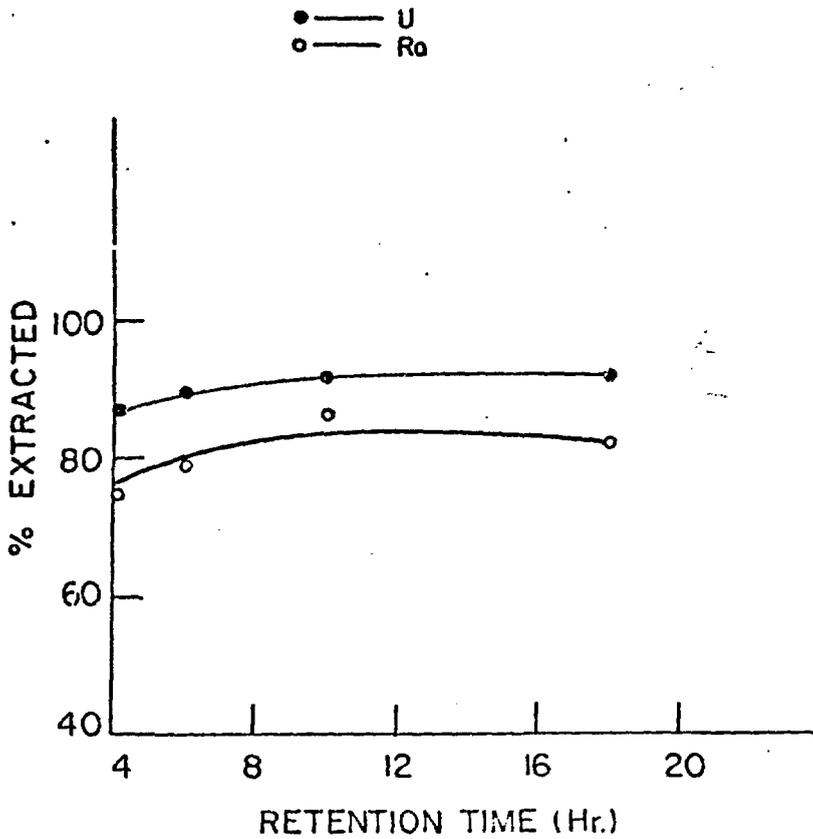
Fig. 3 - Retention time effect on U and Ra extraction
