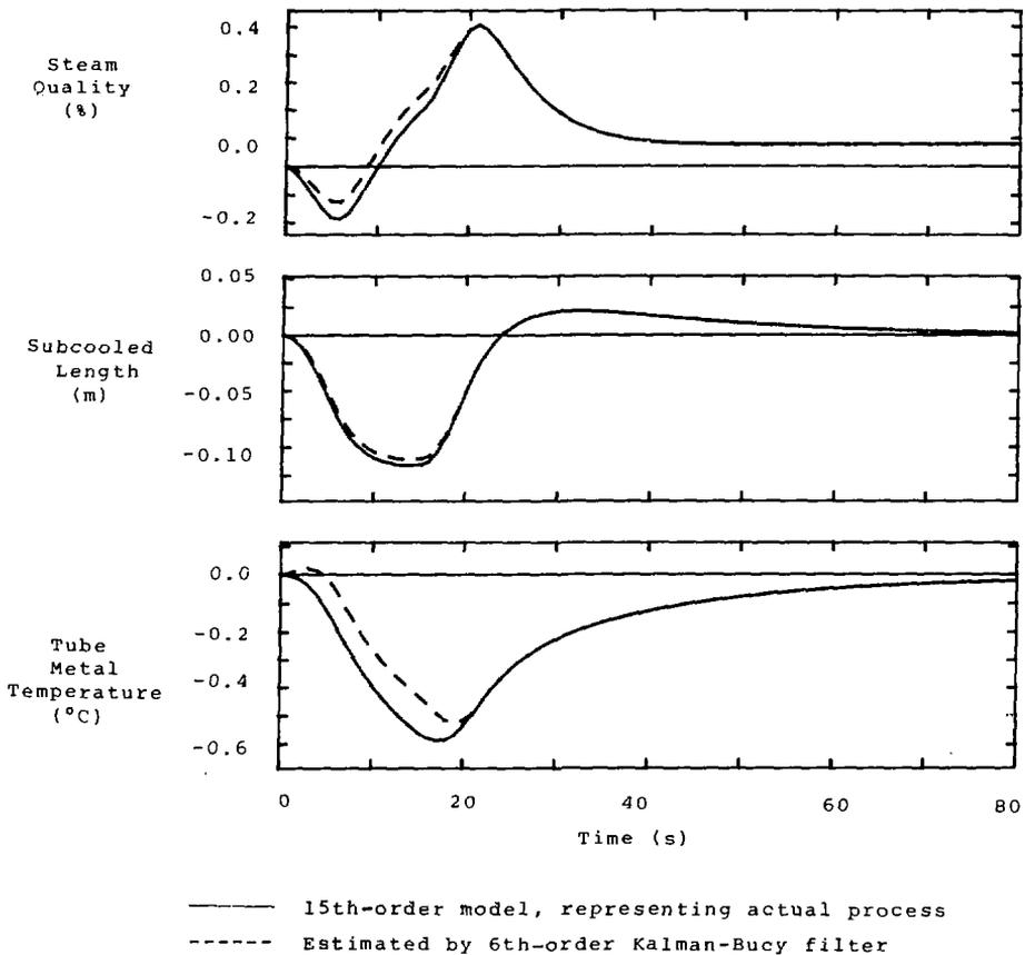
FIGURE 6b COMPARISON OF THE RESPONSES OF THE STEAM GENERATOR MODEL AND THE KALMAN-BUCY FILTER TO A STEAM VALVE DISTURBANCE
