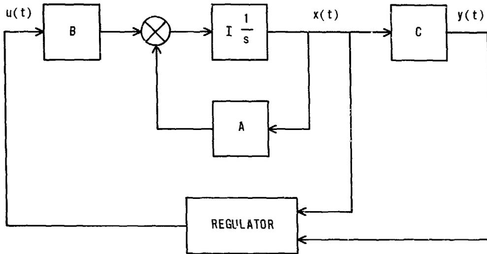
FIGURE 2: TIME - INVARIANT OPTIMAL REGULATOR
