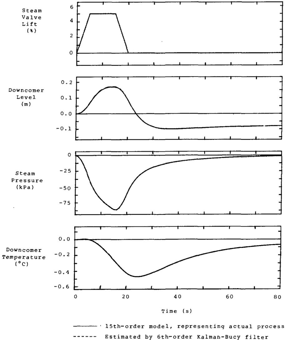
FIGURE 6a COMPARISON OF THE RESPONSES OF THE STEAM GENERATOR MODEL AND THE KALMAN-BUCY FILTER TO A STEAM VALVE DISTURBANCE
