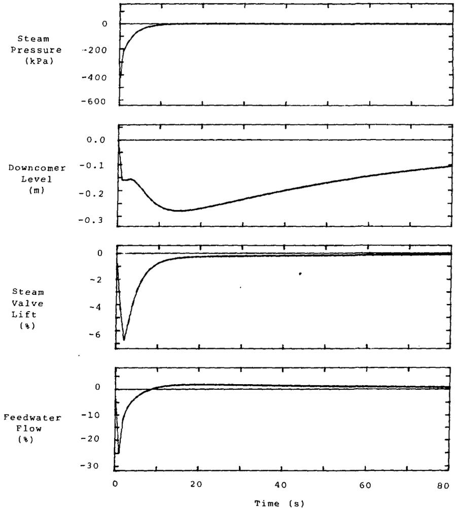
FIGURE 9 RESPONSE OF THE OPTIMAL CONTROLLER TO AN INITIAL PRESSURE DEVIATION WITH THE 6 STATES PROVIDED BY A KALMAN FILTER HAVING INCORRECT INITIAL CONDITIONS
