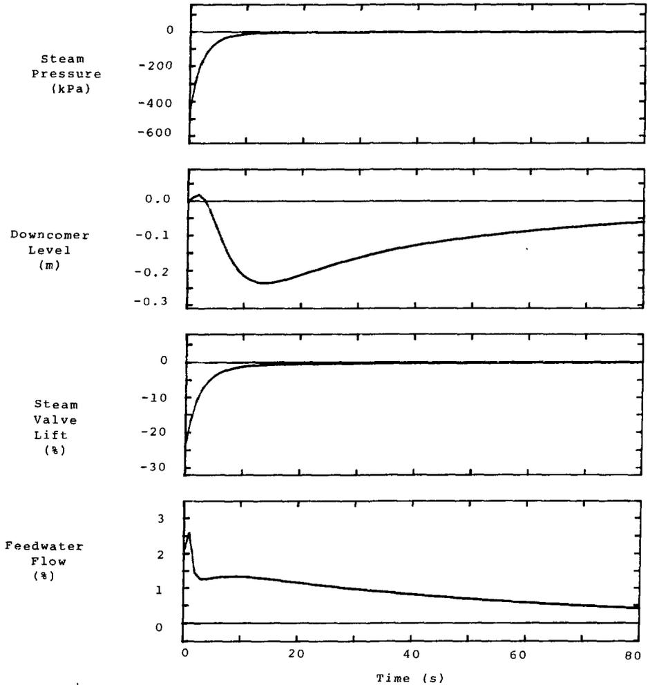
FIGURE 8 RESPONSE OF THE OPTIMAL CONTROLLER TO AN INITIAL PRESSURE DEVIATION WITH THE 6 STATES PROVIDED BY A KALMAN FILTER HAVING THE CORRECT INITIAL CONDITION
