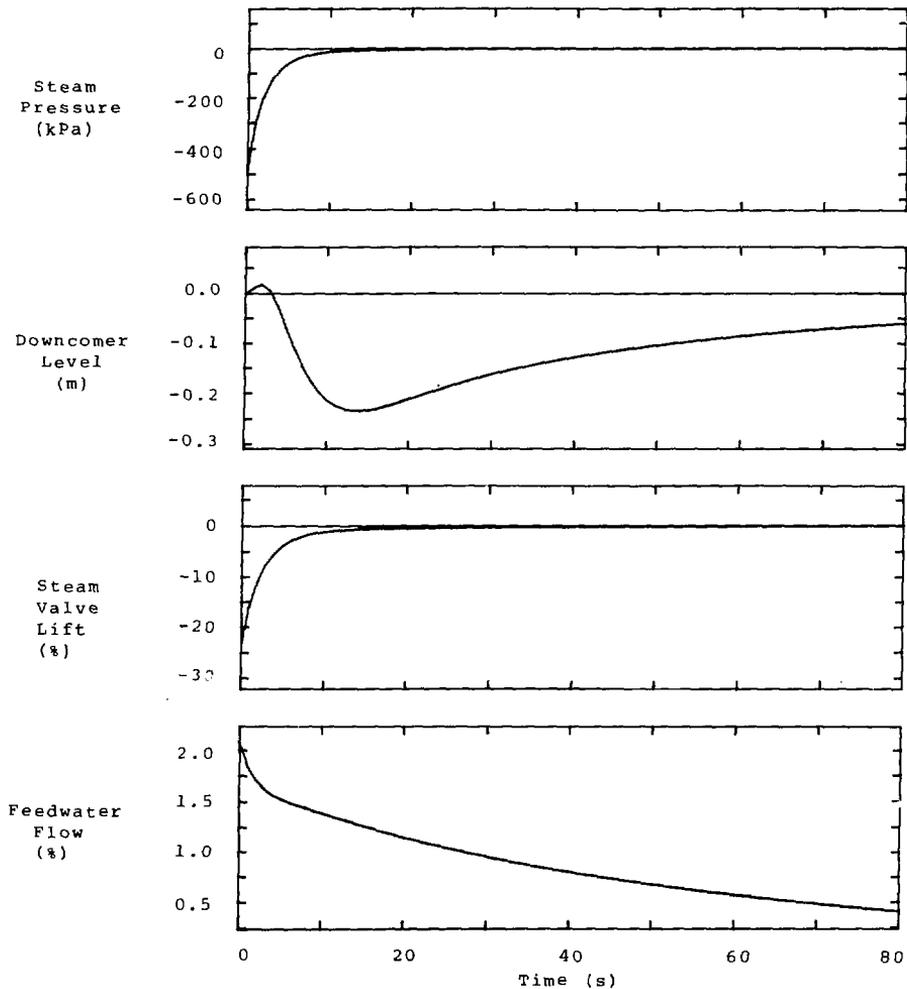
FIGURE 7 RESPONSE OF THE OPTIMAL CONTROLLER TO AN INITIAL PRESSURE DEVIATION, WITH THE 6 STATES PROVIDED BY THE MODEL
