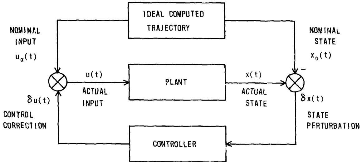
FIGURE 1: OPTIMAL CONTROLLER STRUCTURE
