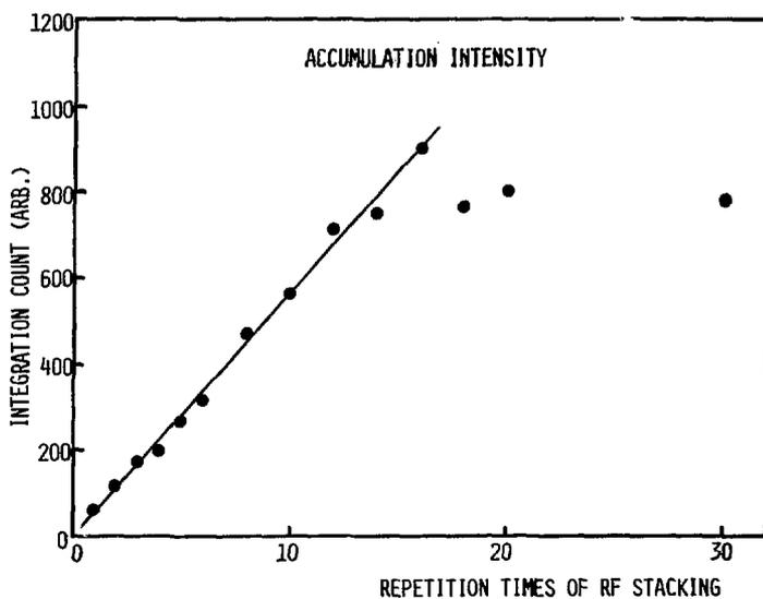
Fig. 11. Beam accumulation intensity versus the repetition times of RF stacking.
