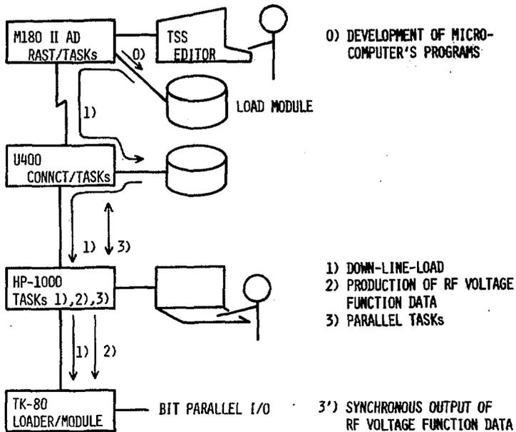
Fig. 4. Microcomputer's software development system with M180 II AD and task execution form HP-1000.
