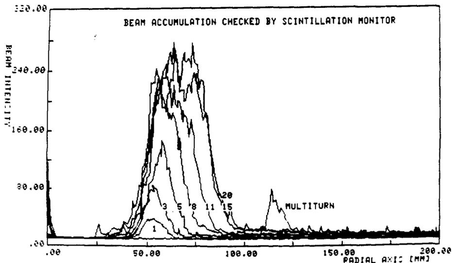
Fig. 10. Beam profile of the stacked beam.
