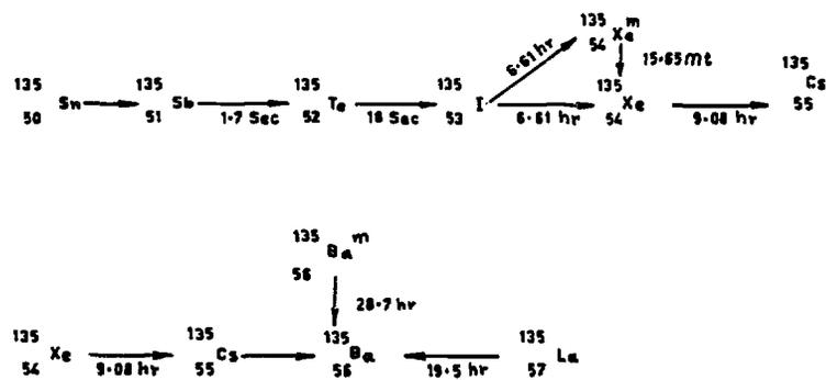
FIG. 2. EXPANDED XENON DECAY CHAIN
