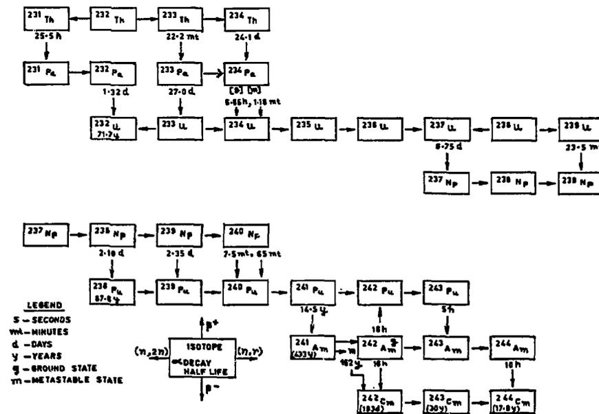
FIG. 1. DEPLETION AND BUILDUP CHAINS OF ACTINIDES
