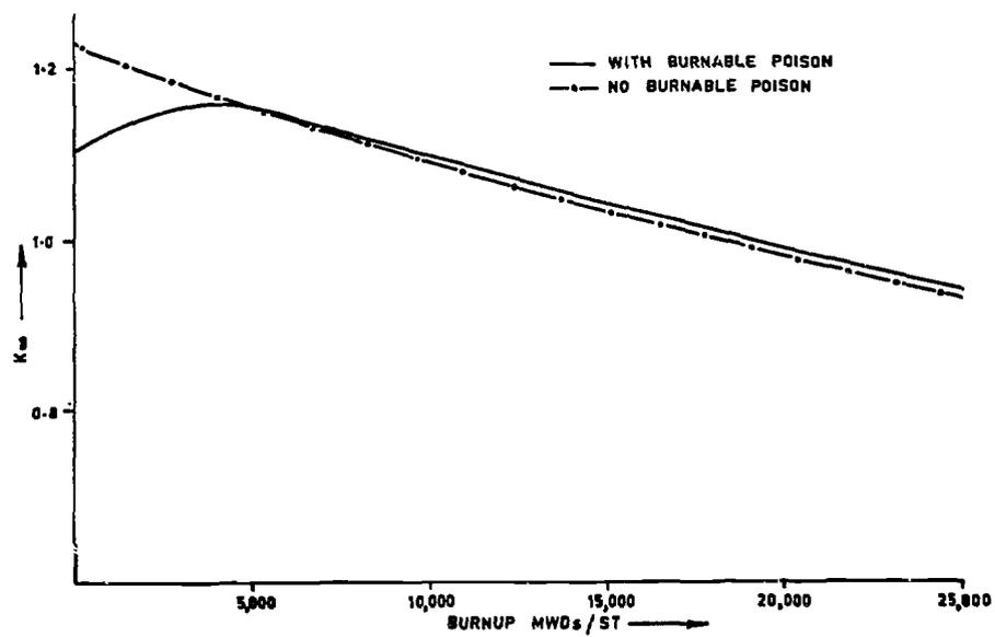
FIG. 4.  $K_{\infty}$  VARIATION WITH BURNUP FOR A BWR FUEL BUNDLE WITH AND WITHOUT BURNABLE POISON (IN CHANNEL VOID FRACTION = 0.4)
