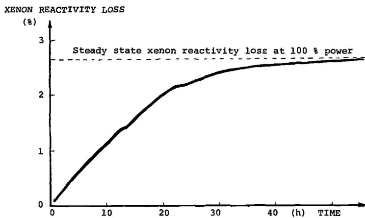
314 2.2.4 Figure 4 EXAMPLE OF REACTOR START-UP FROM XENON FREE CONDITION
