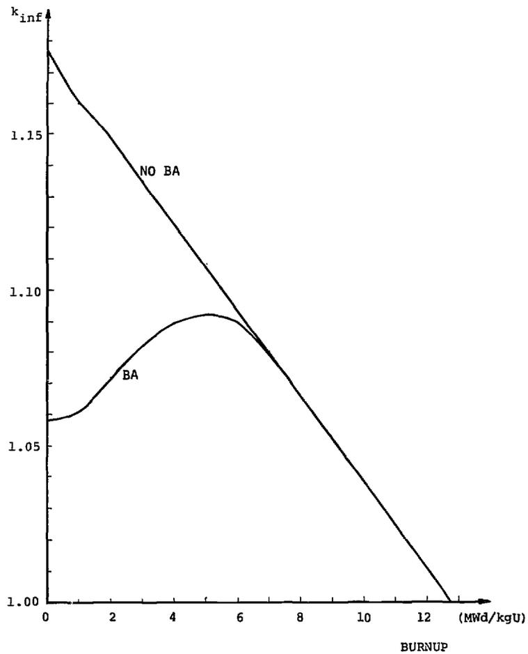
2.2.4  $K_{INF}$  AS A FUNCTION OF BURNUP FOR FUEL WITH AND WITHOUT BA
