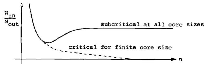
The method is valid as long as the core composition remains uniform and is applicable even for rather large subcritical reactivities. In practice, the minimum in the curve is not always clearly distinguished but most important is the trend towards a constant ratio for the large core.
