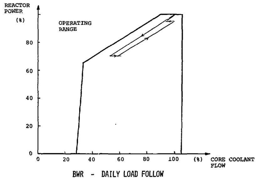
2.2.4 Figure 5 EXAMPLE OF POWER REDUCTION TO 70% WITH USE OF RE-CIRCULATION PUMPS AT CONSTANT CONTROL ROD PATTERN
