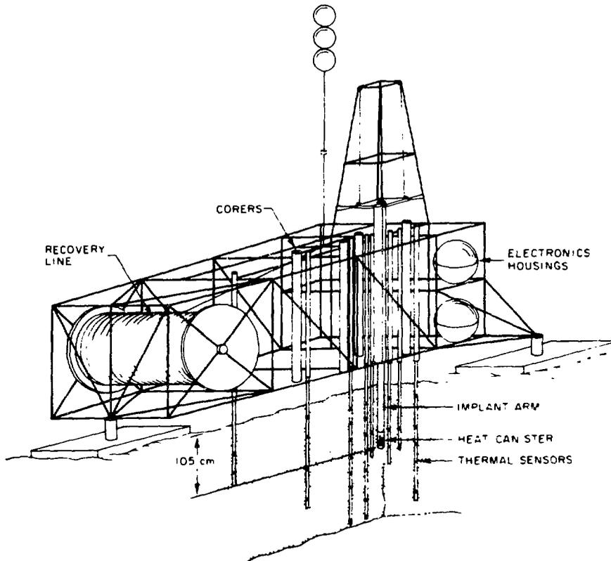
*Platform for an In-Situ Heat Transfer Experiment (ISHTE) planned by the NEA Seabed Working Group to provide data on heat effects on sub-seabed sediments, and develop deep sea experimental technology (Sandia Laboratories, USA).*
