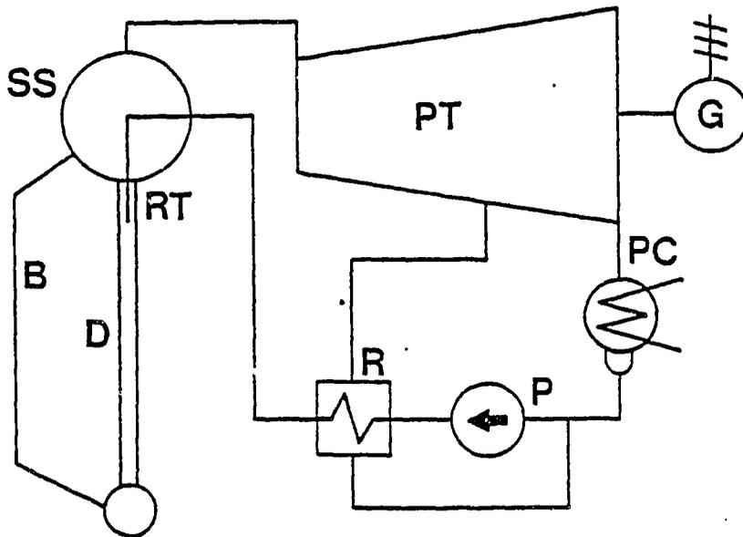
FIG. 3: Simplified Flow Scheme of the Potassium System
