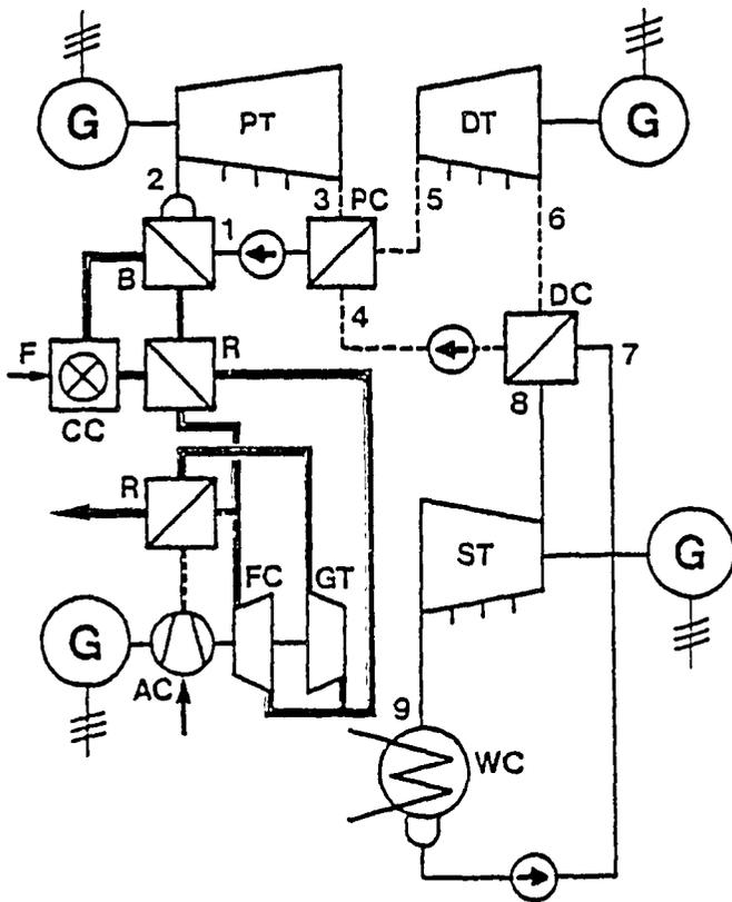
FIG.2a: Simplified Flow Scheme of a "Treble Rankine Cycle"
