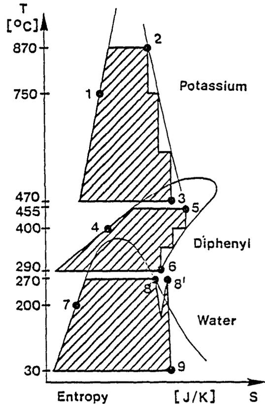
FIG.2b: Temperature-Entropy Diagram of a "Treble Rankine Cycle"
