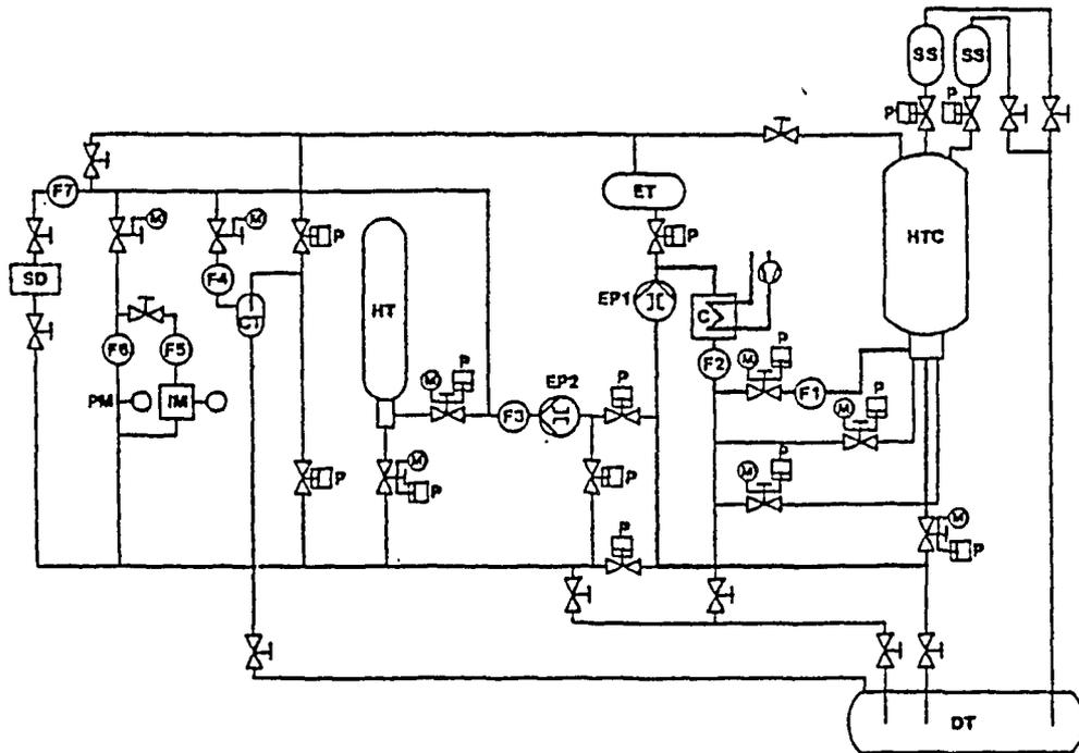
FIG. 4: Simplified Flow Scheme of the Potassium High Temperature Loop "HT 3"
