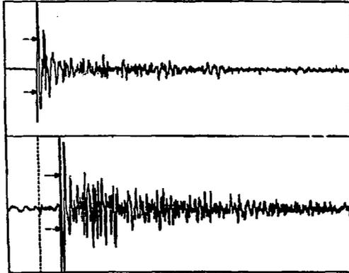
Figure : 19 - DIGITIZED ACOUSTIC EMISSION SIGNALS
