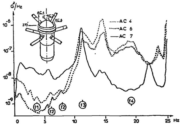
FIGURE 23a : BUGEY 2 - AF30 OF ACCELEROMETERS LOCATED ON TOP COVER HEAD - 2/21/79 - 100 S PP
