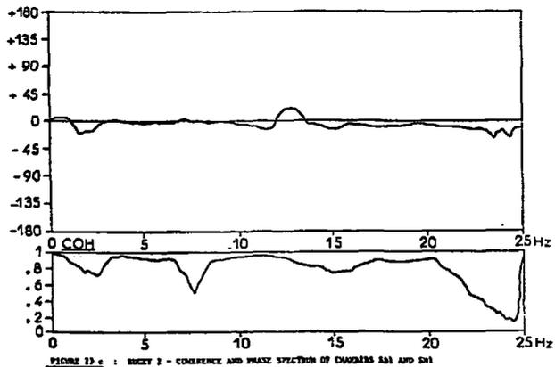
Vibration analysis of the reactors built by Framatome during the past few years, which utilize accelerometers and neutron noise signals, provides experimental confirmation of resonant frequencies and modes of internals predicted by the SAFRAN program.
