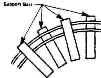
FIG. 15 ELBOW TUBE SUPPORT CONCEPT
