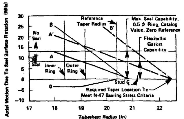
FIG. 7 SEAL MOTION AS A FUNCTION OF RELIEF TAPER LOCATION DOUBLE O-RING CONFIGURATION
