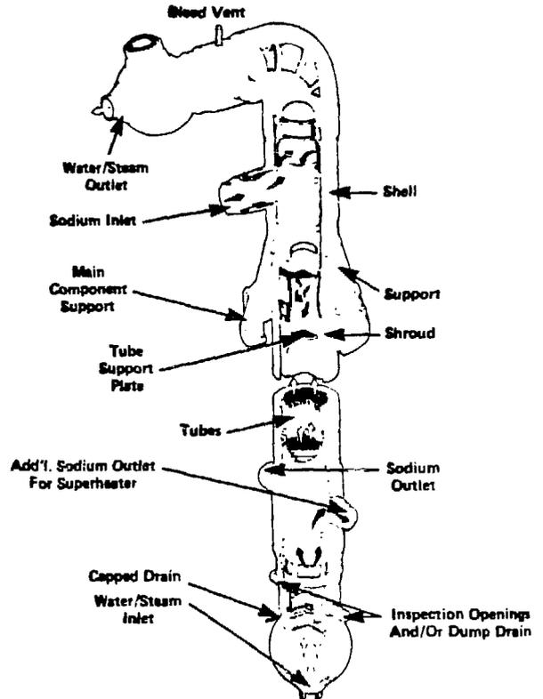
FIG. 3 CRBRP STEAM GENERATOR - PLANT UNIT
