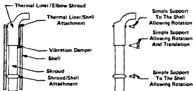
FIG. 9 BASIC CONCEPT OF INTERNAL STRUCTURE SUPPORT
