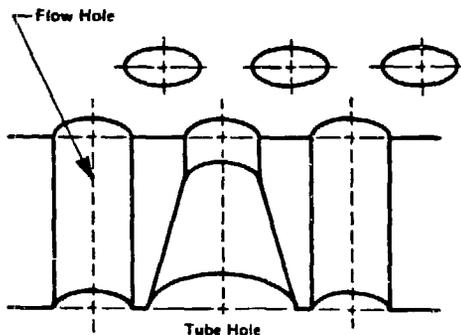
FIG. 14 TUBE HOLE GEOMETRY
