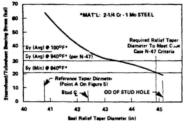
FIG. 6 SEAL SURFACE BEARING STRESS AS A FUNCTION OF RELIEF TAPER DIAMETER (200klb/Bolt Pre-load Double O-Ring)
