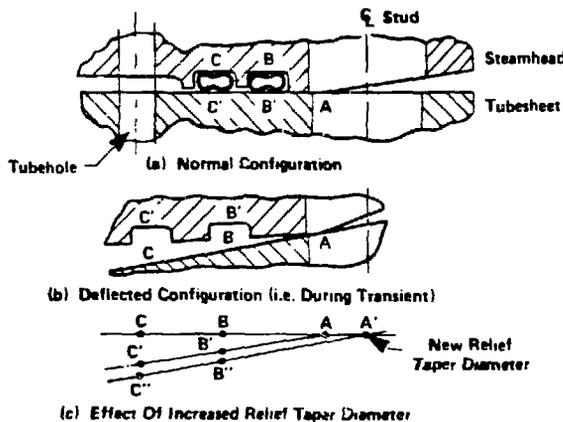
FIG. 5 SEAL ROTATION AS A FUNCTION OF RELIEF TAPER DIAMETER
