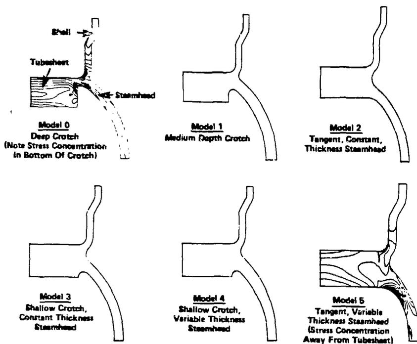
FIG. 8 INTEGRAL STEAMHEAD/TUBESHEET CONCEPTS
