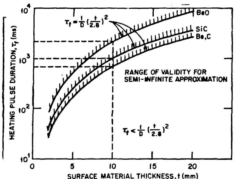
Fig. 2. Range of validity for semi-infinite slab approximation
