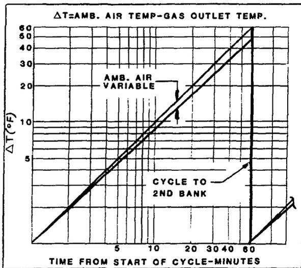
Fig. 4. Vaporizer performance (data provided by Thermax, Inc., South Dartmouth, Massachusetts).
