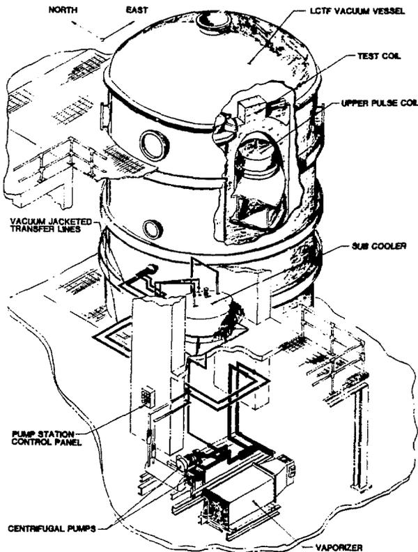
Fig. 2. LCTF at ORNL with PCCS equipment.
