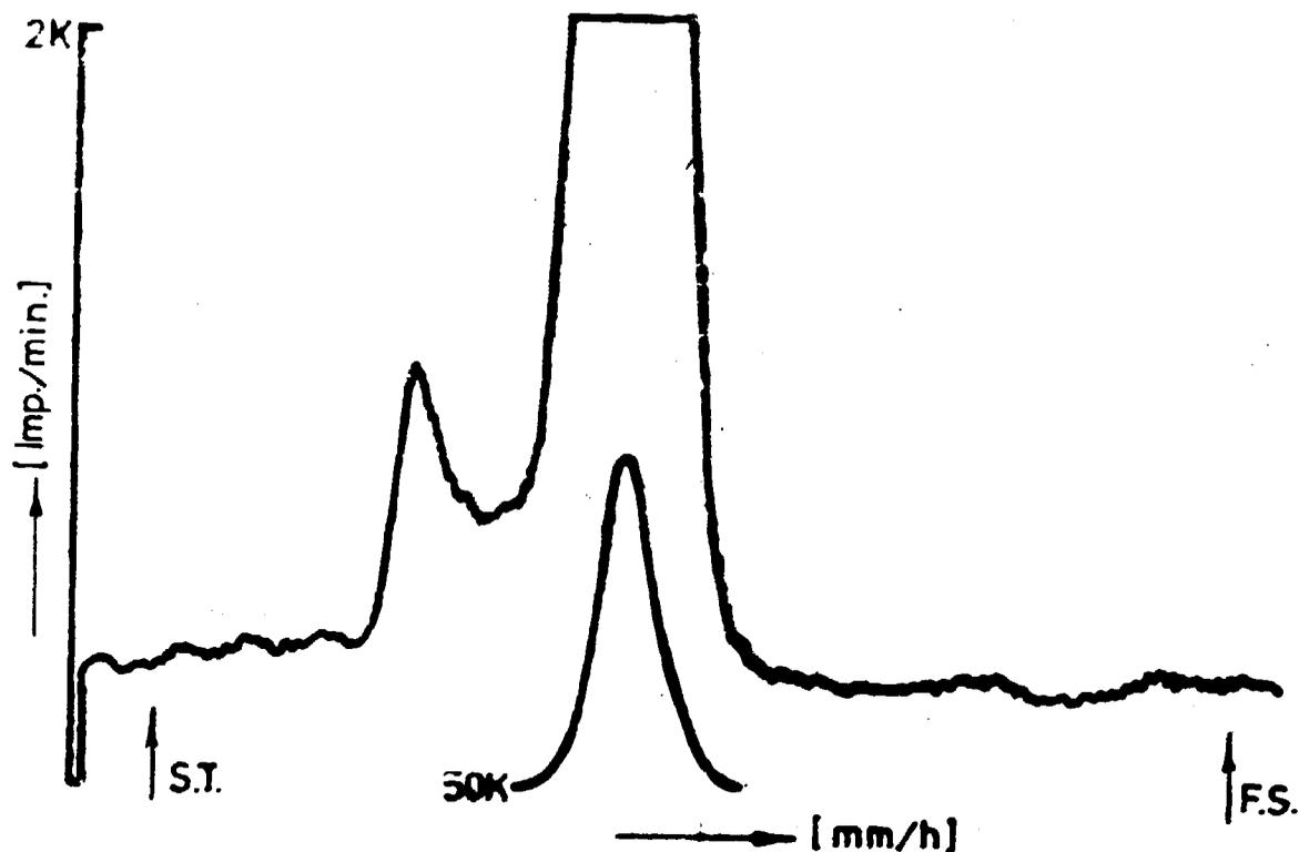
**Figure 7** : Partition chromatography of hydrocortisone. Mobile phase: chloroform ; stationary phase: dimethyl formamide; radiochemical purity : 95,7% ;  $R_F$  hydrocort. =  $0.43 \pm 0.05$ .
