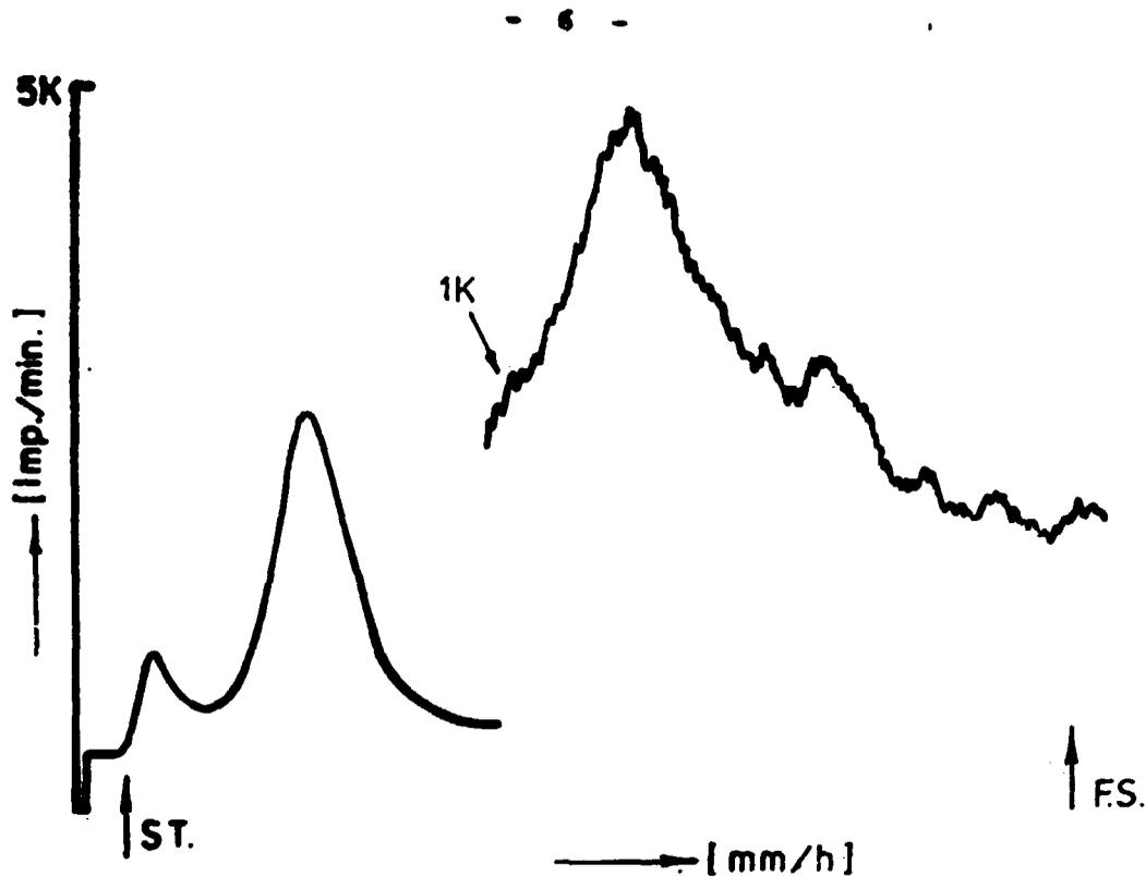
**Figure 6** : Double development of chromatogram; stationary phase: Silicagel G<sub>F</sub> ; mobile phase: chloroform - acetone ( 4 : 1 v/v ).
