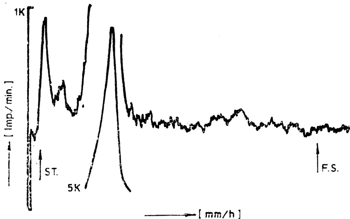
Figure 2 : Stationary phase: Silicagel G<sub>P</sub>; mobile phase : methylene chloride - acetone ( 4:1 v/v ); R<sub>F</sub> hydrocort. 0.214; radiochemical purity : about 84%.
