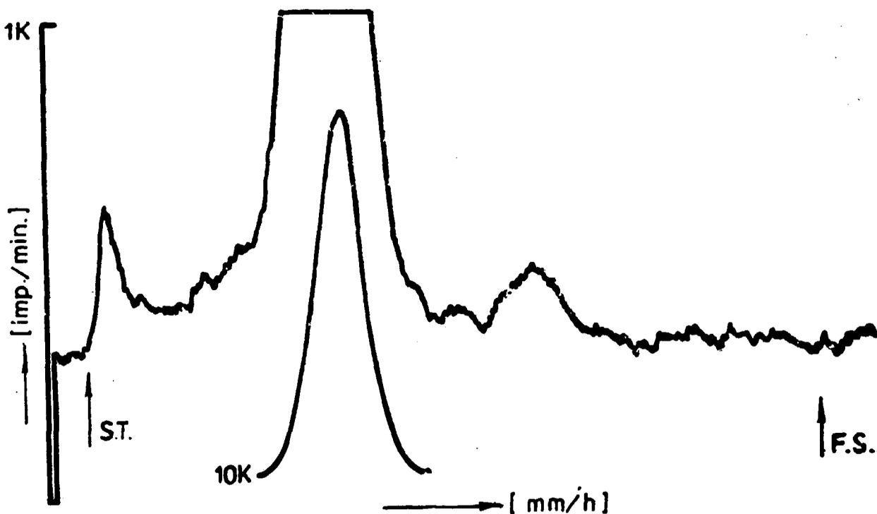
**Figure 1** : Stationary phase : Silicagel G<sub>F</sub> ; mobile phase: chloroform-acetone ( 2:1 v/v ) ; R<sub>F</sub> hydrocort. : 0.356; radiochem. purity: 91.5%.
