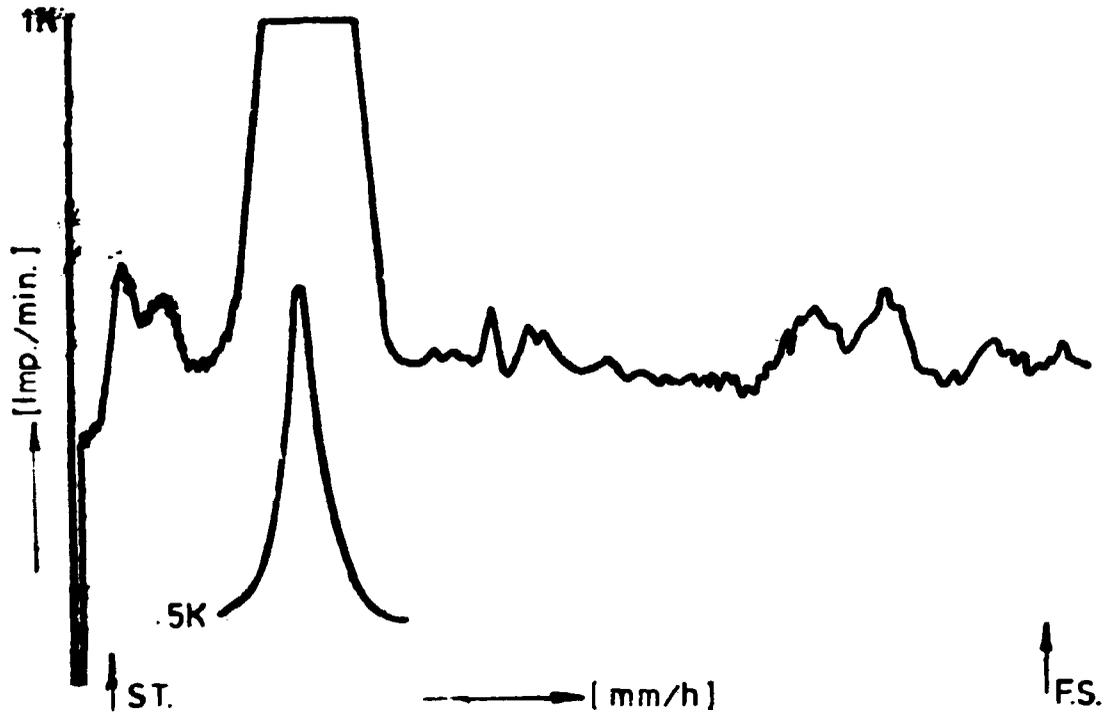
**Figure 4 :** Addition of inactive carrier; stationary phase: Silicagel  $G_p$ ; mobile phase: methylene chloride-acetone ( 4 : 1 v/v ).
