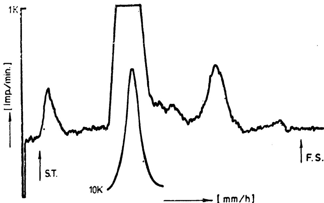
Figure 3 : Stationary phase : Silicagel G<sub>P</sub>; mobile phase : chloroform-absolute ethenol - water (9:1:0.1 v/v); R<sub>F</sub> hydroc. 0.355; radiochem. purity : 85%.
