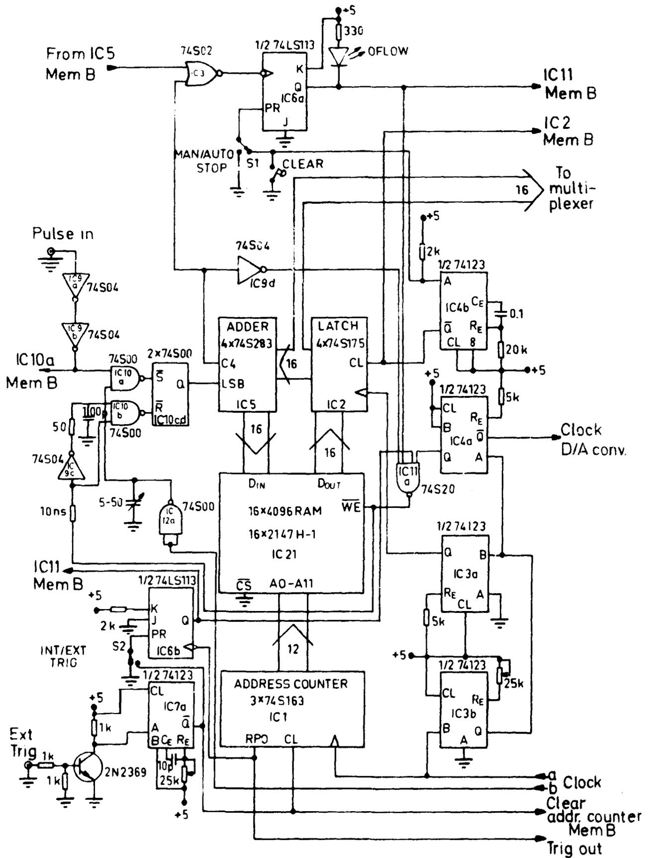
Fig. 4 Circuit diagram of the memory, arithmetic unit, address counter and control circuits
