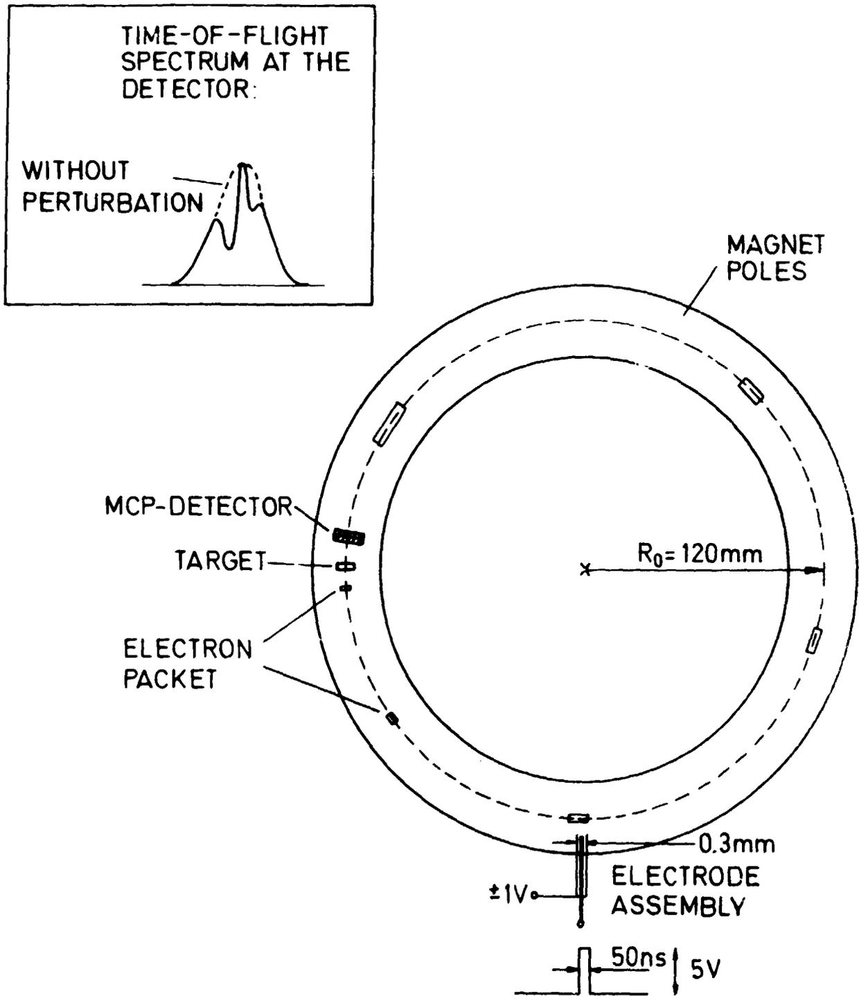
Fig. 8 Top view of the time-of-flight electron spectrometer drawn schematically. The same electron packet is shown in different parts of the flight path.
