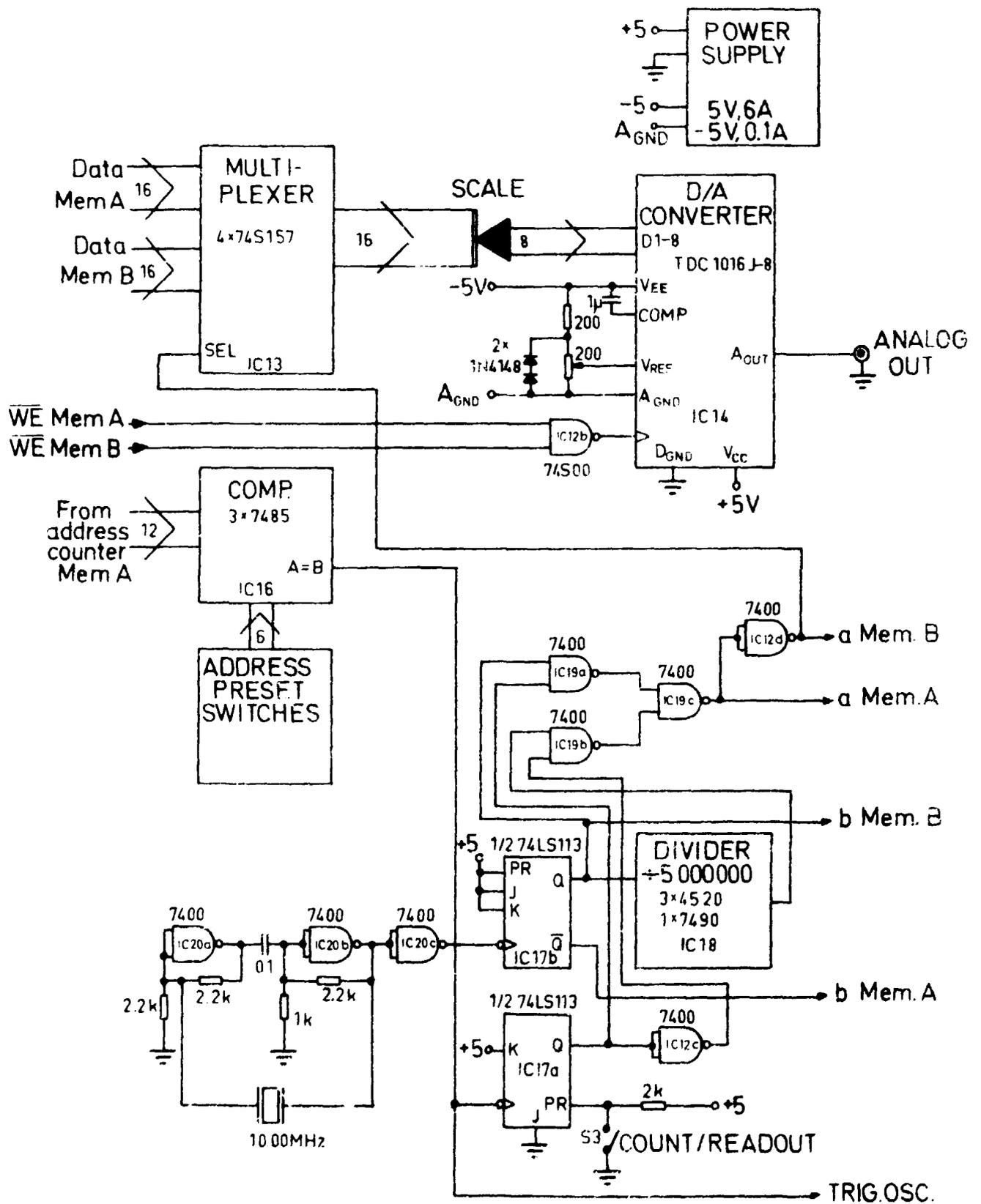
Fig. 6 Clock and output circuits
