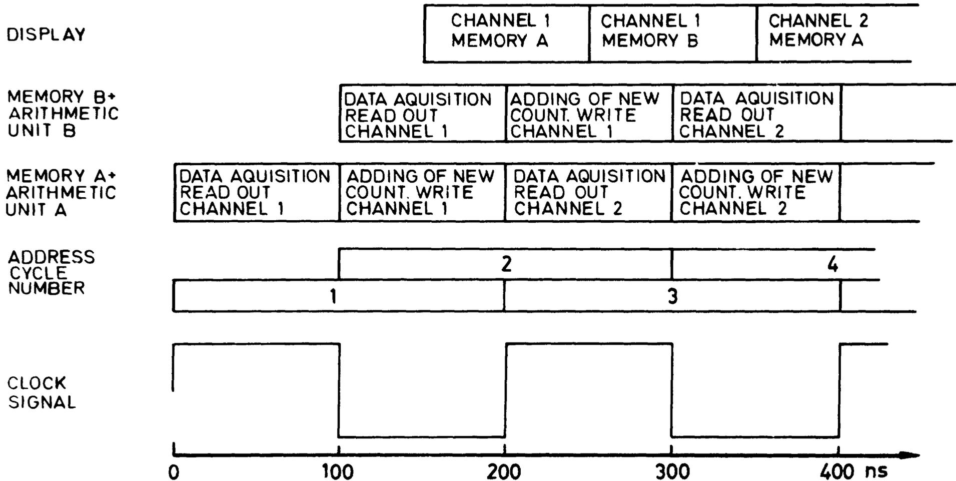
Fig. 3 Clock signal and address cycles of the memories
