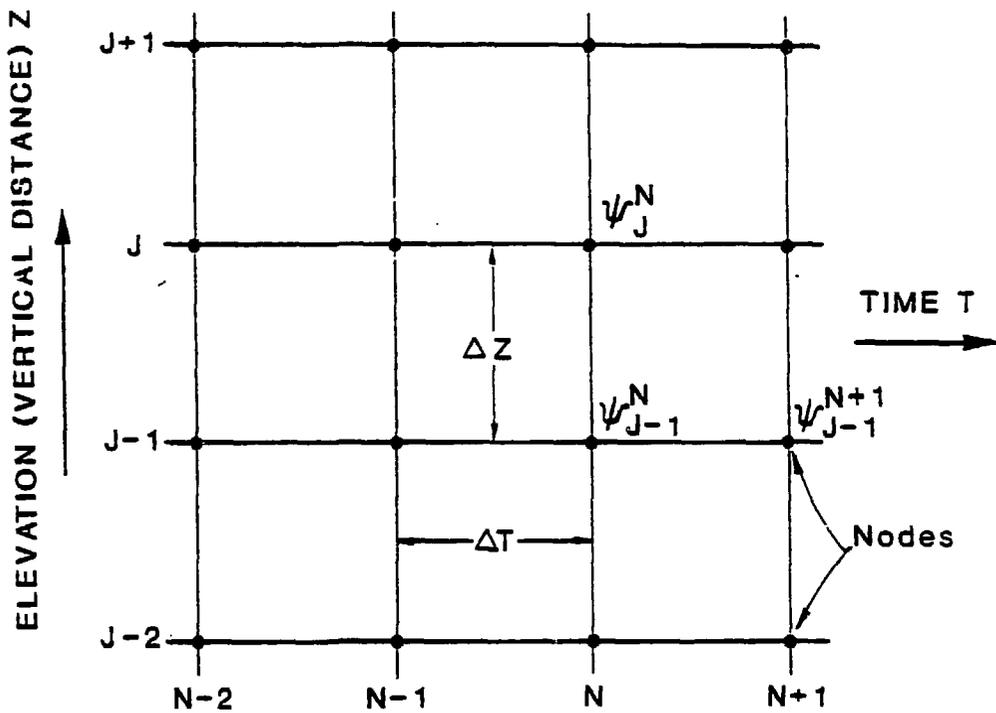
Figure 3. Two Dimensional Net Representing the Space and Time Coordinates ( $\psi_J^N$  represents the Pressure Head at Node  $J$  in the Time Step  $N$ ).
