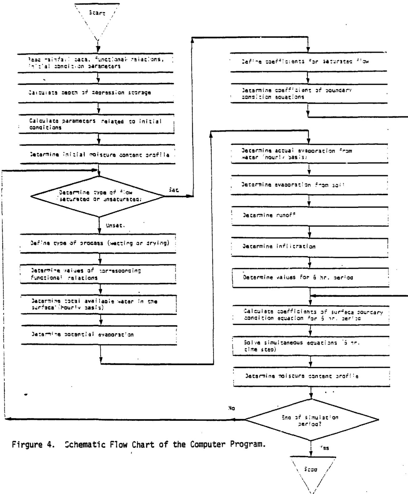
Figure 4. Schematic Flow Chart of the Computer Program.
