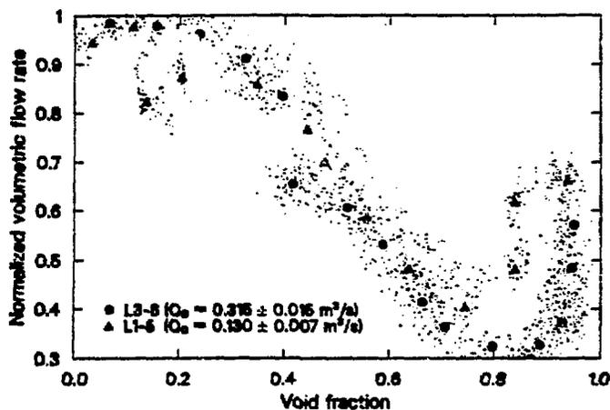
Fig. 5 Normalized pump volumetric flow rate
