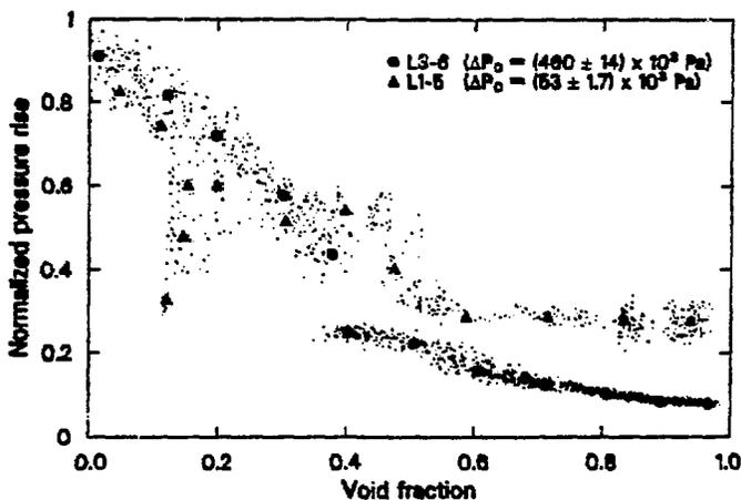
Fig. 3 Normalized pressure-rise across the pump
