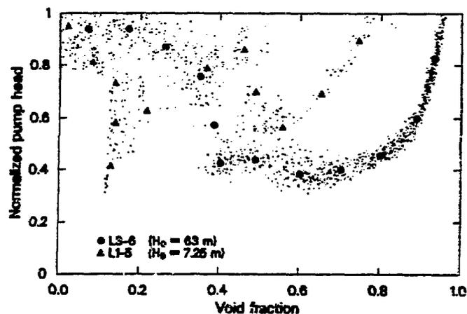
Fig. 8 Normalized pump head
