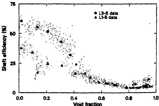
Fig. 11 Pump shaft efficiency
