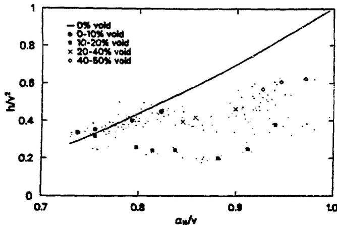
Fig. 12 L1-5 two-phase head vs. single-phase head (HVN)
