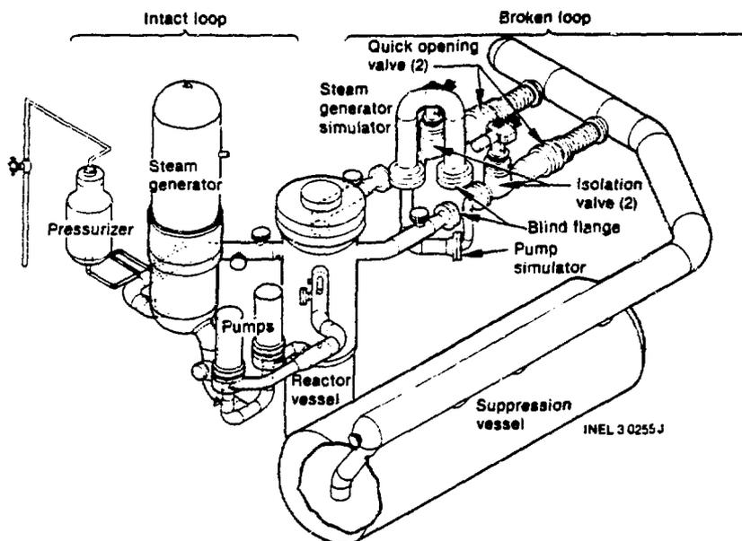
Fig.1 Axonometric projection of LOFT system
