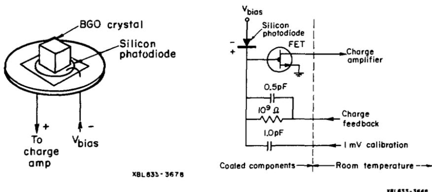
Figure 4: (a) Schematic of  $3 \times 3 \times 3 \text{ mm}^3$  BGO crystal mounted on a Hamamatsu R1722-01 silicon photodiode with 4 mm diameter photosensitive area. Crystal was polished, cemented to photodiode with RTV and coated with MgO powder. (b) Schematic of cooled components of the scintillator, photodiode and charge amplifier.
