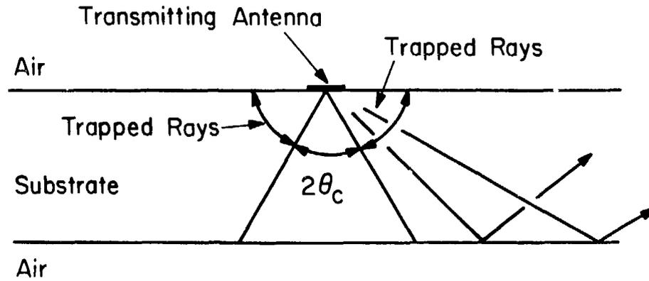
Fig. 2 Ray picture of excitation of trapped surface waves on a substrate. Substrate rays outside the wedge  $2\theta_c$  are completely reflected and trapped as surface waves. The critical angle ( $30^\circ$ ) shown is appropriate for fused quartz ( $\epsilon_r = 4$ ).
