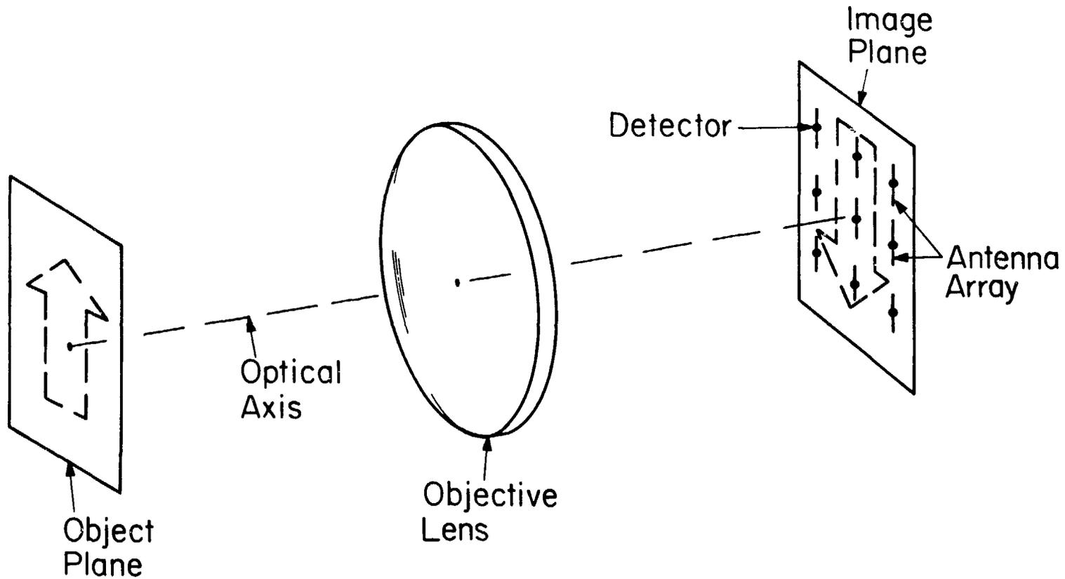
Fig. 1 Imaging with an array of antennas with individual detectors at the image plane.
