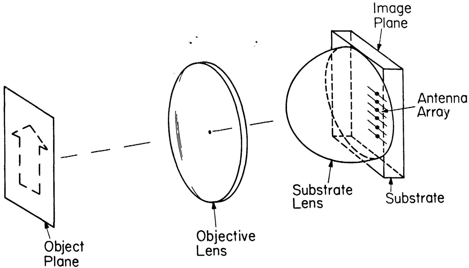
Fig. 6 Substrate-lens coupled antenna array. The substrate lens has been added to the system of Figure 1.
