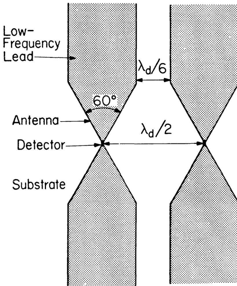
Fig. 7 Modified bow-tie for an imaging antenna array.
