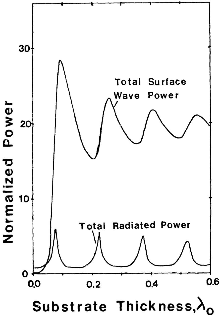
Fig. 4 Calculated distribution of power radiated by a short slot in a ground plane on a substrate with a dielectric constant of 12. Power is normalized to the power the same slot would radiate in free space. Surface waves dominate for thicknesses greater than  $\lambda_0/20$ .
