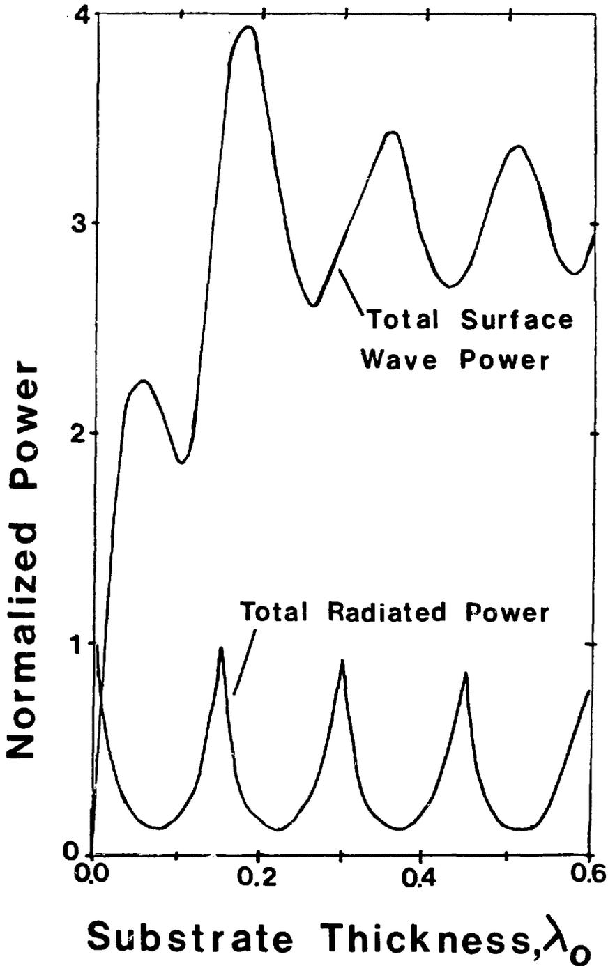
Fig. 3 Calculated distribution of power radiated by a short dipole on a substrate with a dielectric constant of 12. Power is normalized to the power the same dipole would radiate in free space. Surface waves dominate for thicknesses greater than  $\lambda_0/100$ .
