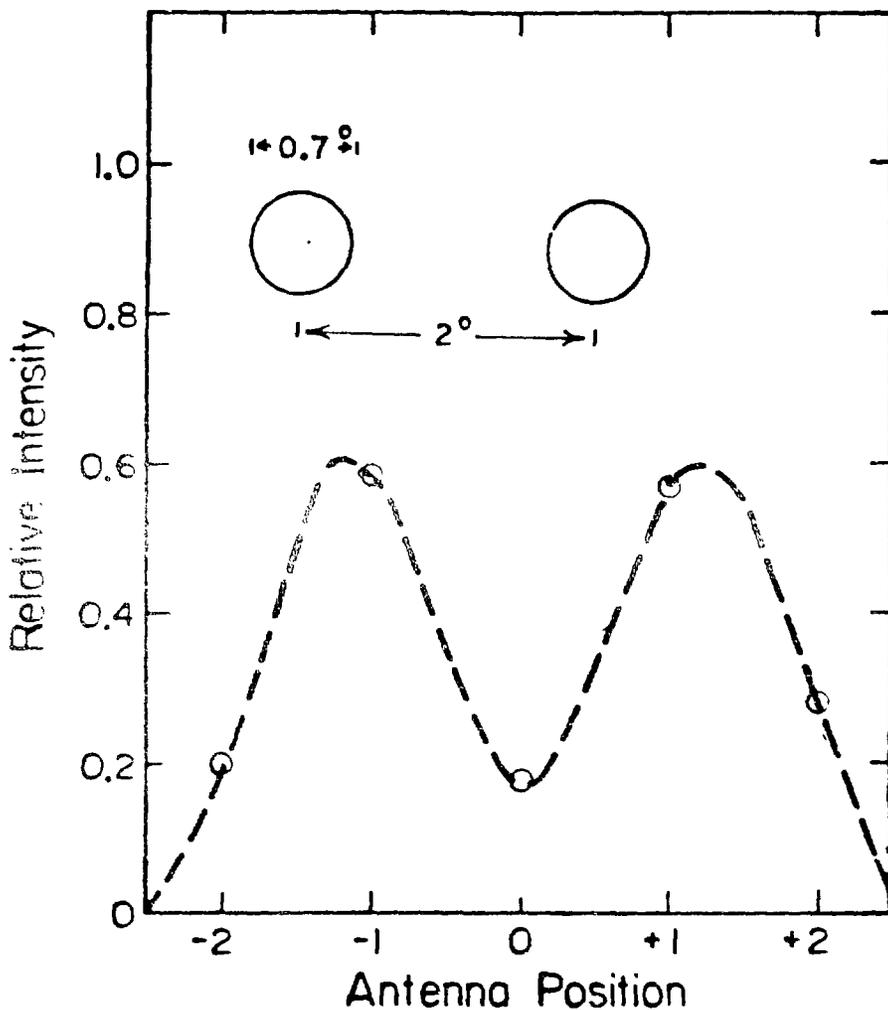
Fig. 10 Measured array images of two pinholes at 1.2 mm. The separation between the pinholes is 20% larger than the Rayleigh limit. The open circles are the observed signals. Points between the sampled values were recovered by the standard sinc-function interpolation of sampling theory (16, pp. 21-22).
