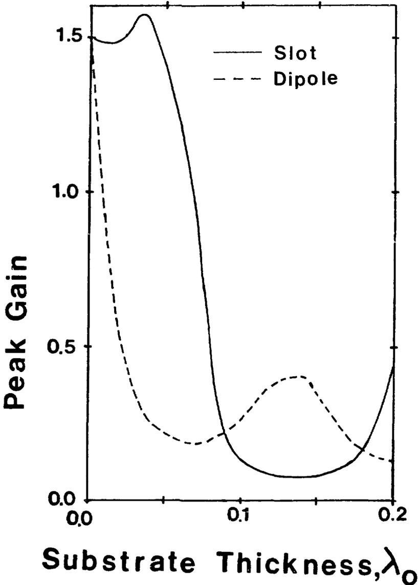
Fig. 5 Calculated peak gain of short slots and dipoles on substrates with a dielectric constant of 12. The direction for peak gain is down through the substrate. The slot gain rolls off quickly for thicknesses greater than  $\lambda_0/20$ . The substrate lowers the dipole gain even for thin substrates.
