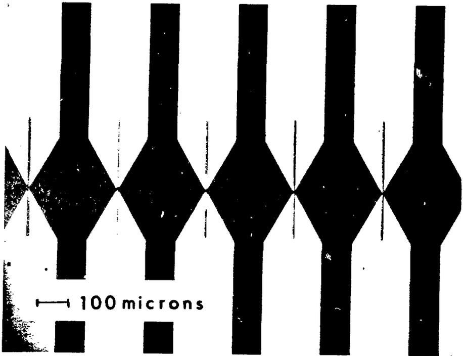
Fig. 8 Bow-tie array for a wavelength of 1.2 mm. The bow arms are evaporated silver and the substrate is fused quartz. The narrow line that crosses the gap between the arms of the bow is evaporated bismuth. The microbolometer is formed where the bismuth crosses the gap.
