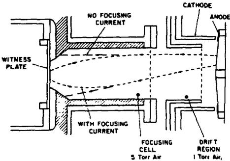
Fig. 8. Final focusing experiment mounted on front of Gamble II diode.
