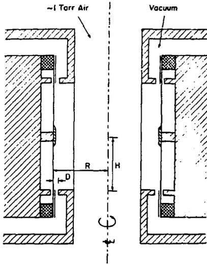
Fig. 3. Equitorial-pinch-reflex diode.
