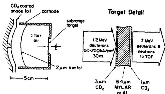
Fig. 4. Experimental set up for energy-loss measurements.
