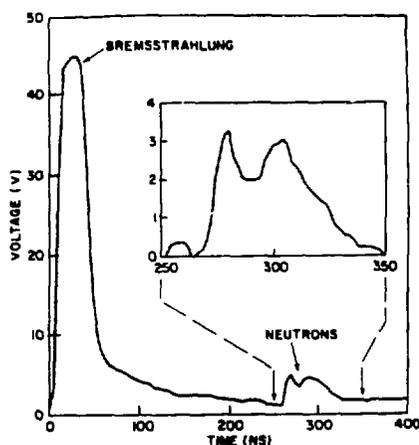
Fig. 5. Neutron TOF trace for Mylar stopping foil, spherical diode and 7.6 m flight path.
