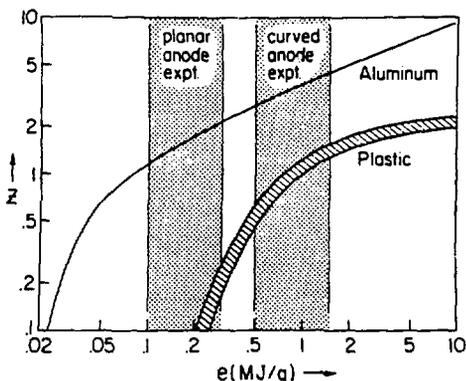
Fig. 7. Average ionization state ( $\bar{z}$ ) versus internal energy density ( $e$ ) for aluminum and plastic ( $\text{CH}_2$ ).
