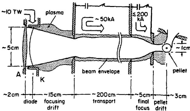
Fig. 1. Schematic of modular Light-Ion ICF system.
