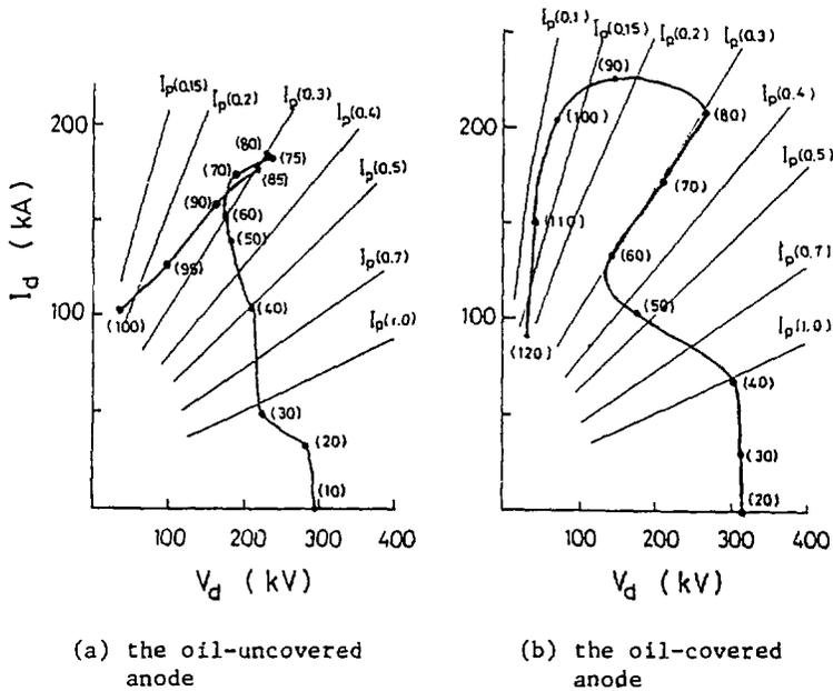
Fig.3.  $V_d$ - $I_d$  diagrams. (t) is time in ns, and  $I_d$  is the parapotential current for the effective gap  $d$  in cm.
