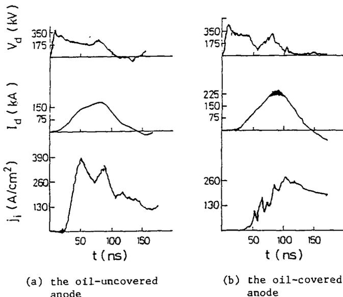
Fig.2. Typical oscilloscope traces of the diode voltage  $V_d$ , the diode current  $I_d$  and the ion current  $j_i$ .
