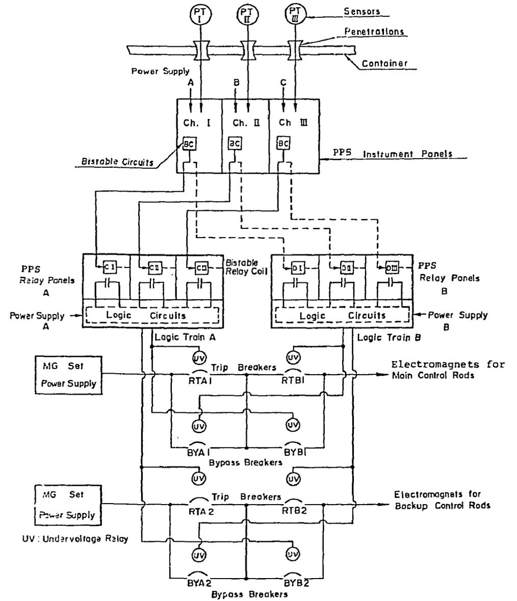
Fig. 3-5 Plant Protection System Instrumentation
