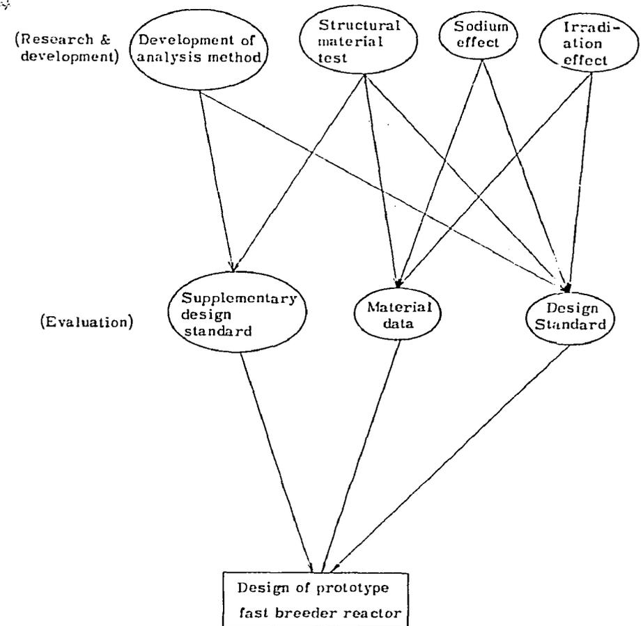
Fig. 11-2 Research and Development of Structural Materials and Their Reflection on the Design of Fast Breeder Reactor
