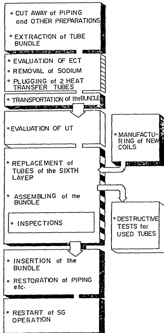
Fig. 7-2 Maintenance and Repair Test Items on 50MW SG Test Facility
