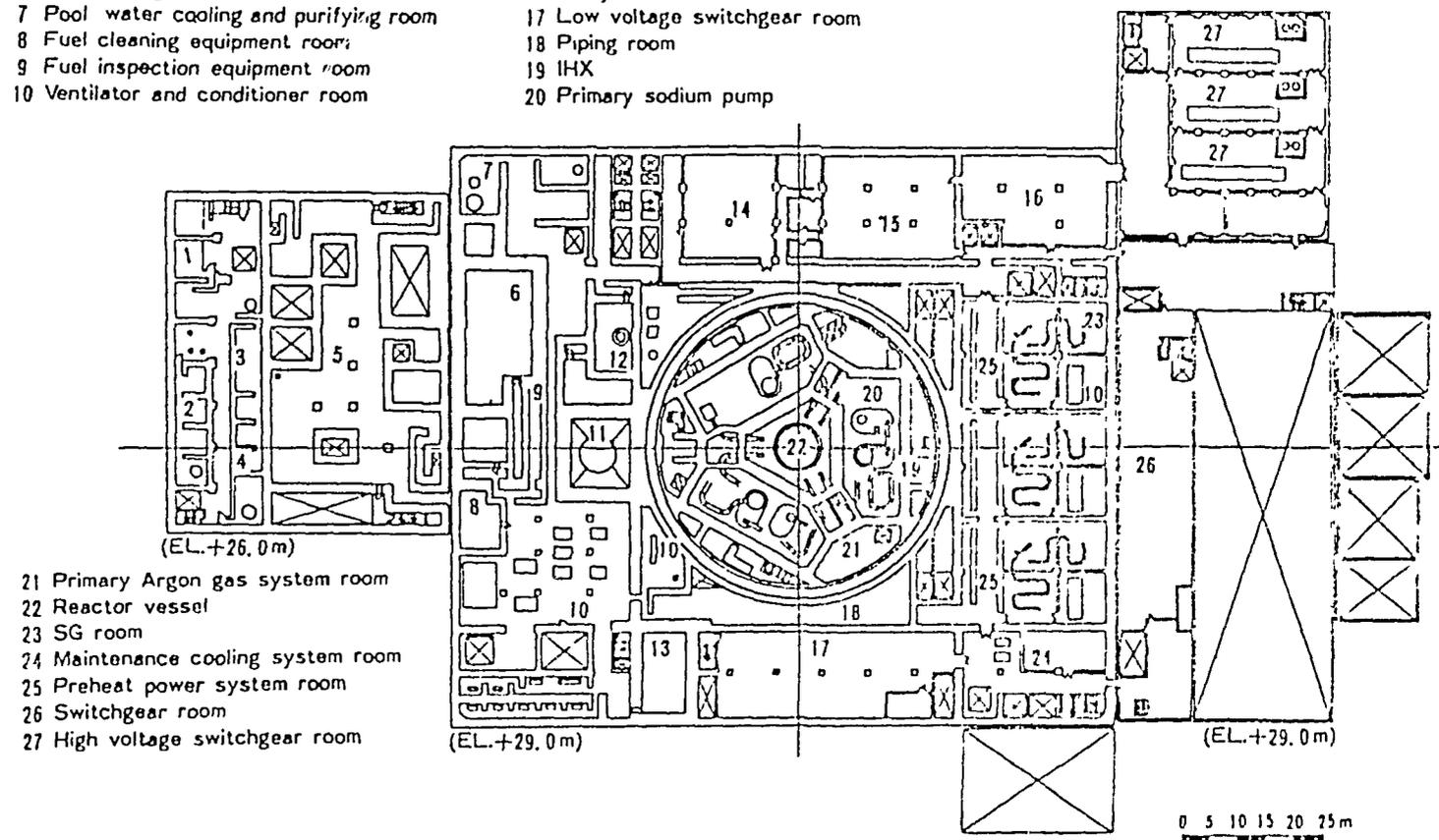
Fig. 3-8 Horizontal Cross Section of Main Buildings
