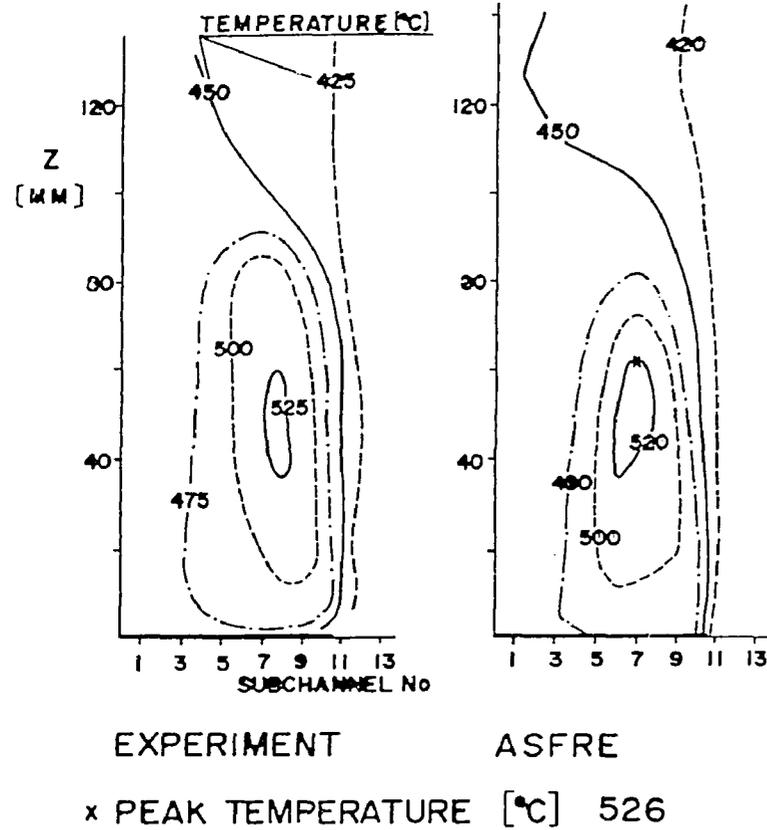
Fig. 12-1 Benchmark Calculation 49% Central Blockage
