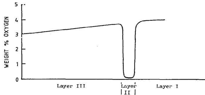
FIG. 13 ELECTRON IMAGE AND OXYGEN DISTRIBUTION FOR FUEL ROD HEATED AT 1800°C FOR 1 MIN.
