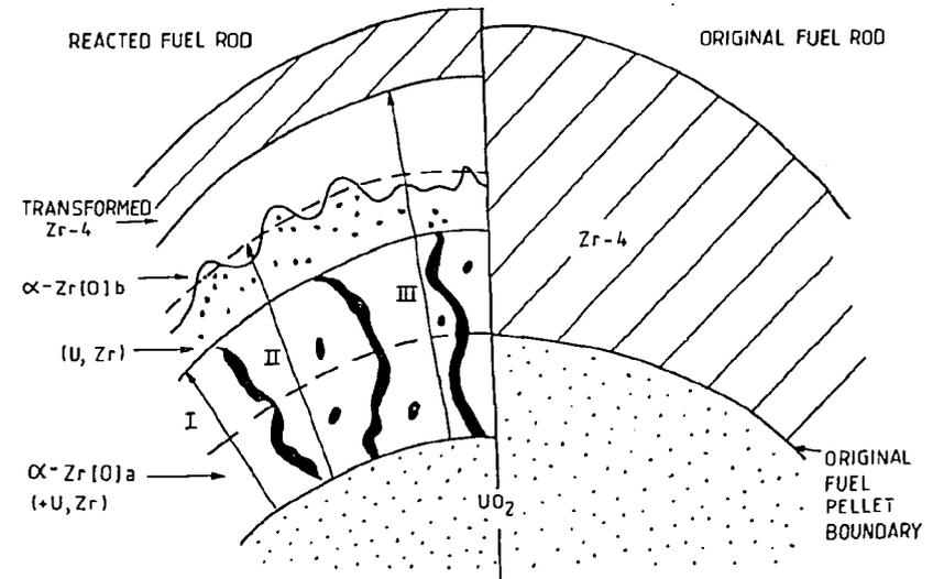
FIG. 3 SEQUENCE OF PHASES FORMED IN THE REACTED ZONE.
