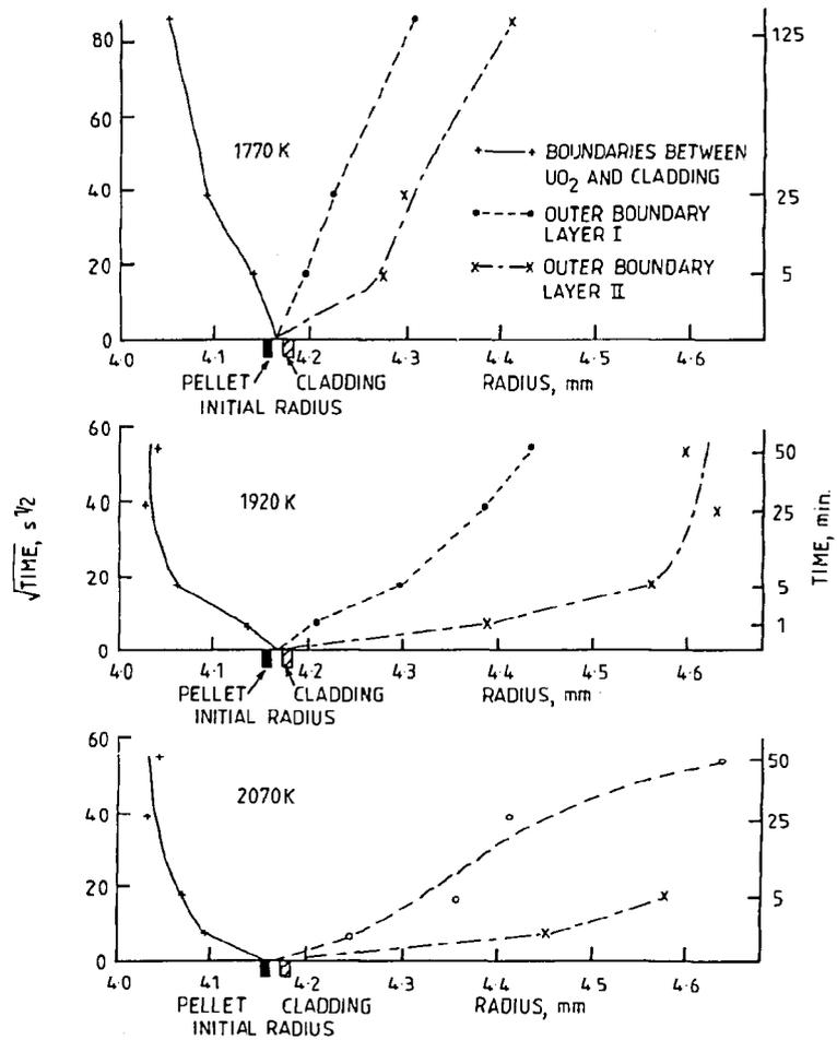
FIG. 7. CHANGE OF LAYER BOUNDARY RADIUS WITH TIME
