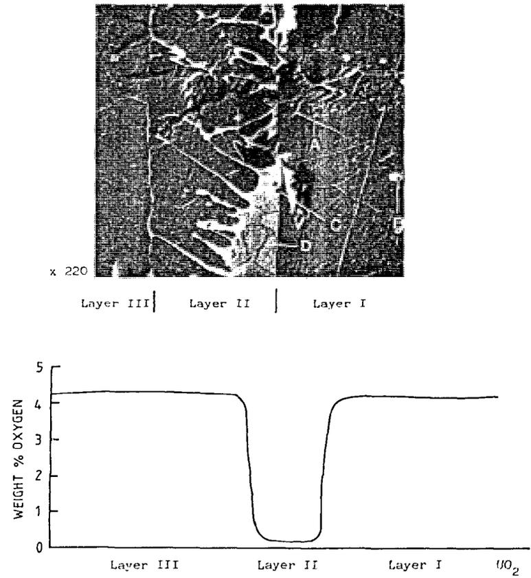
FIG. 12 ELECTRON IMAGE OF THE U/Zr ZONE AND OXYGEN DISTRIBUTION IN A FUEL ROD HEATED AT  $1500^\circ C$  FOR 120 MIN.
