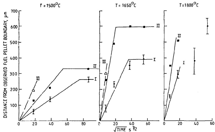
FIG. 9 RATES OF GROWTH OF LAYERS OF REACTION PRODUCTS
