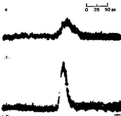
Fig. 2 Longitudinal charge distribution measured by a streak camera for a total charge of  $5 \times 10^{10} e^-$ : (a) no compression, 32 ps FWHM; and (b) same beam with compression (but without scraping), 15 ps FWHM (risetime = 3.3 ps).
