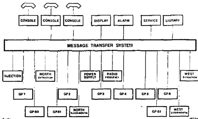
Fig. 2. Single layer architecture at the SPS 1976.
