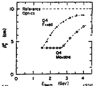
Fig. 3. Energy dependence of  $\beta_y^*$  for the microbeta insertion for SPEAR.
