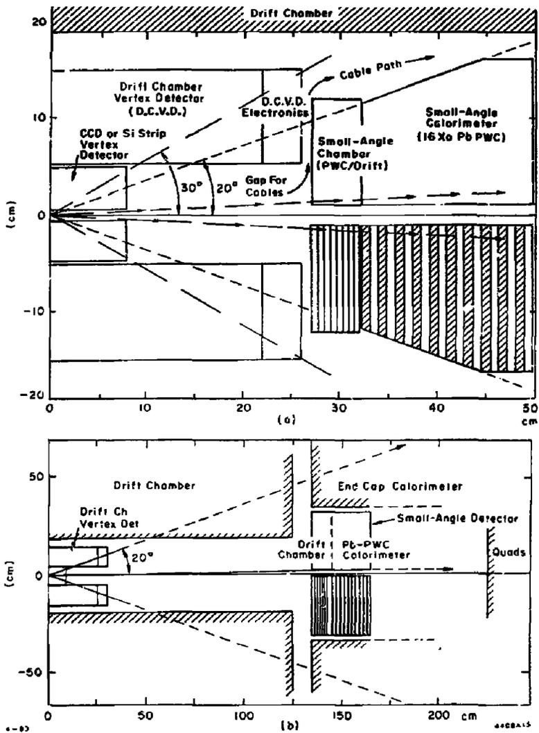
Fig. 13. Two geometries of the portion of the MAKK II detector near the SLC interaction point that are compatible with the two final triplet schemes that have been studied. For the reasons given in the text, the detector will be designed to be similar to the geometry given in (b).
