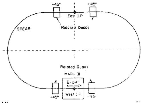
Fig. 9. Locations of the rotated quadrupole magnets that will compensate the effects of the MARK III solenoid.
