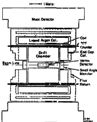
Fig. 12. Side view of the MARK II detector at the SLC.
