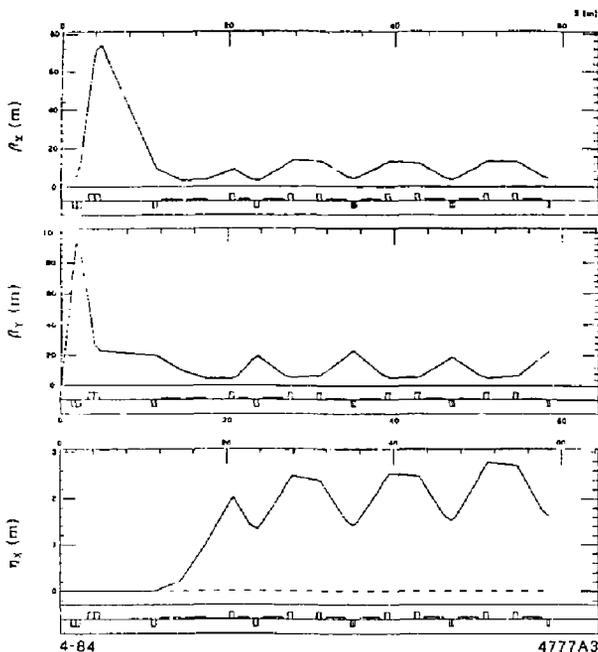
Fig. 8. The beta functions,  $\beta_x$  and  $\beta_y$ , and the dispersion function,  $\eta_x$ , for the minibeta optics ( $\beta_y^* = 3$  cm) plotted as a function of the distance from the interaction point (in meters) along the central trajectory of the SPEAR ring.
