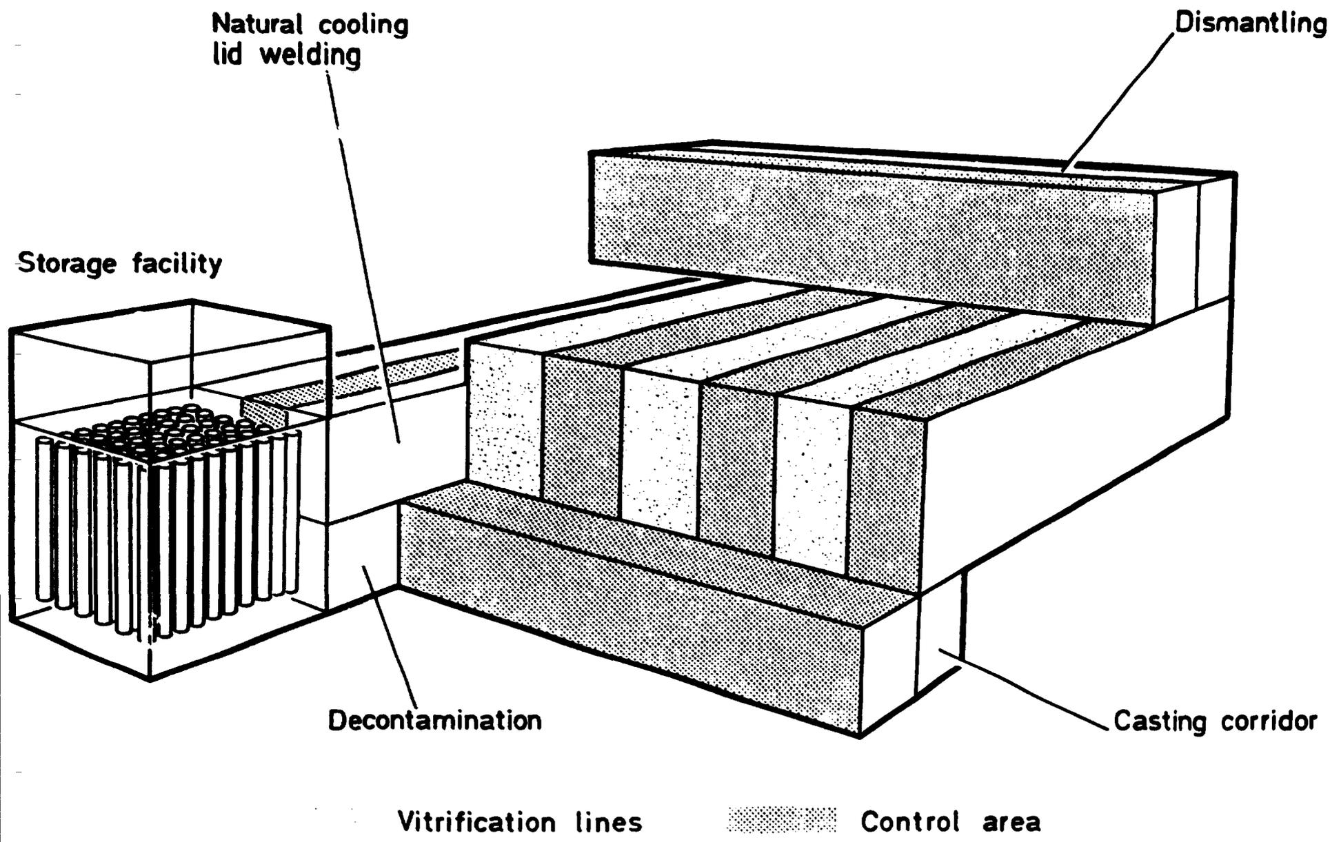
FIGURE 8 : LAY OUT OF THE LA HAGUE VITRIFICATION PLANT (R<sub>7</sub> AND T<sub>7</sub>)
