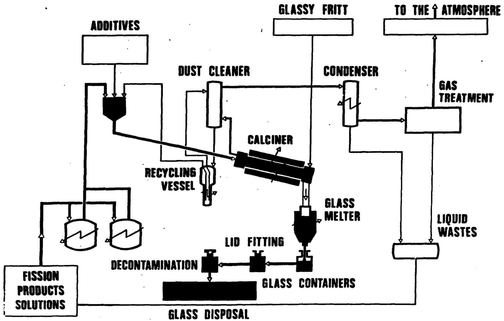
FIGURE 1 : MARCOULE UP1 CONTINUOUS VITRIFICATION PROCESS SCHEMATIC
