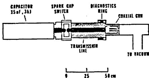
FIG. 1. The compact pulsed accelerator.
